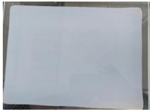
Fast release encapsulant laminated, no delamination
