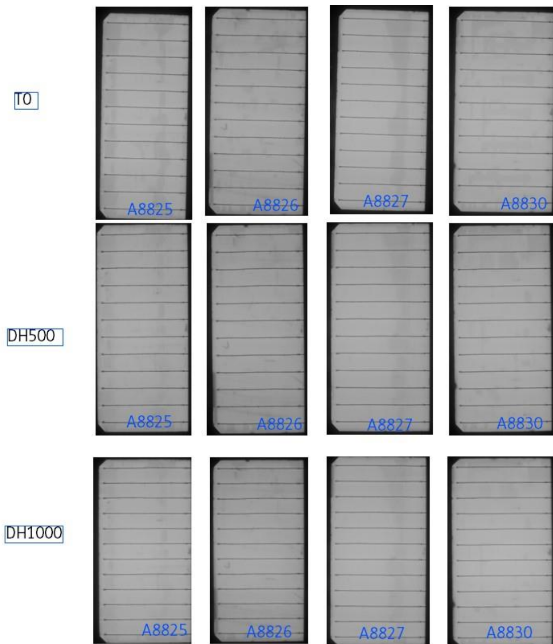
Figure 3.7 Electroluminescence images of a one-cell modules based on fast release encapsulant and re-assembled glass plates at different stages of damp heat testing
