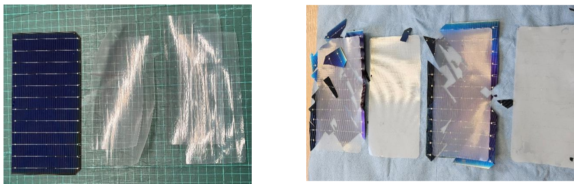
Figure 2.4 Left: Solar cell and release encapsulant before lamination. Right: Solar cells and encapsulant after lamination followed by release/disassembly.
