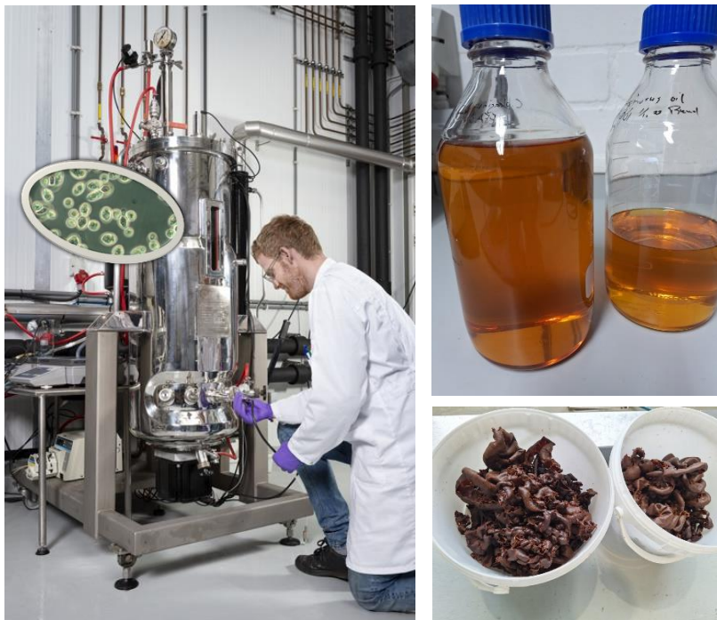
Figure 7 Bioreactor used for fermentation, microorganism and products obtained: oils and defatted biomass. (source: WFBR)
