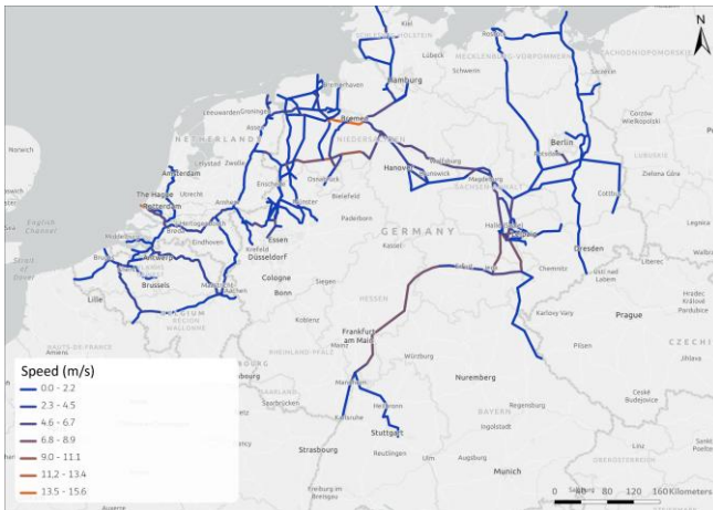
Figure 3.29 Velocity distribution throughout the 2030 network at the moment of maximum flow.
