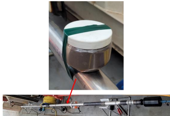
Figure 7 Cup filled with steel shot did not disturb the magnetometer signal in the Directional Module.
