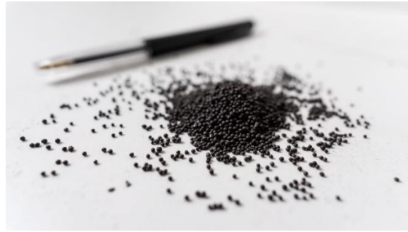
Figure 1 The spherical steel shot particles - diameter 0.6 to 1.2 mm. Picture by Tessa Veldhorst De Schaapjesfabriek©.
