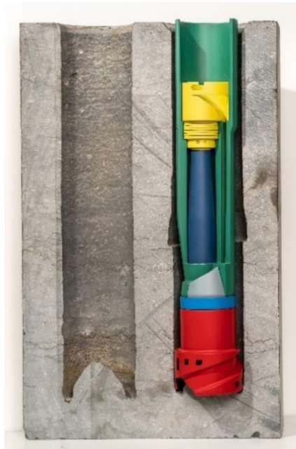
Figure 2 Holes drilled in limestone with a steel shot jet bit. On the right hand side a model of the drill bit including the down hole recirculation device as invented by Shell. Note the high bore hole wall quality. Picture by Tessa Veldhorst De Schaapjesfabriek©.
