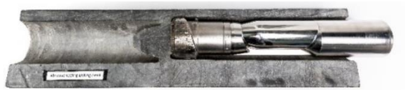
Figure 3 Prototype 2.9 inch steel shot jet bit and drilled holes in Belgian limestone. Picture by Tessa Veldhorst De Schaapjesfabriek©.
