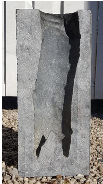
Figure 5 A 4-1/8 inch diameter borehole in Belgian limestone. The hole was drilled with a steel shot jet bit, and steered by erosion based differential hole making
