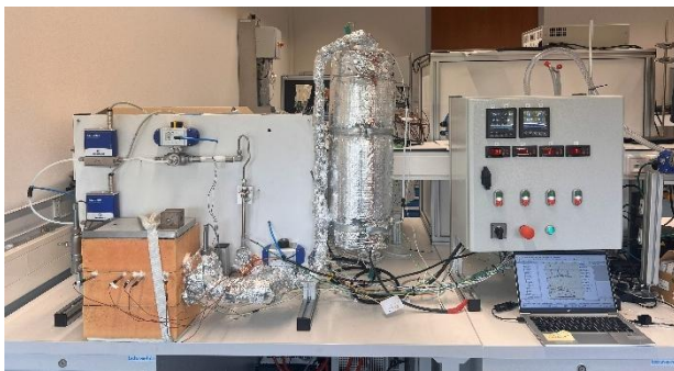
Figure 9. Schematic of the open atmospheric reactor used to characterize the sorption performance of the salt hydrates.
