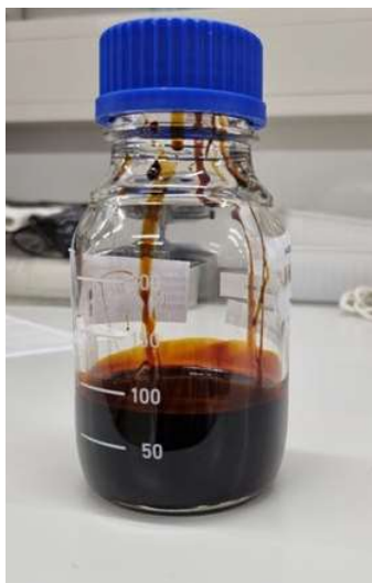
Figure 1 Picture of the first lignin oil sample obtained by catalytic depolymerization and C-alkylation of herbaceous lignin
