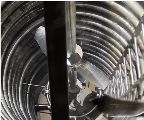
Figure 2. View for the top sight glass of the 15 m 3 fermenter in Grenzach used for the pilot evaluation.
