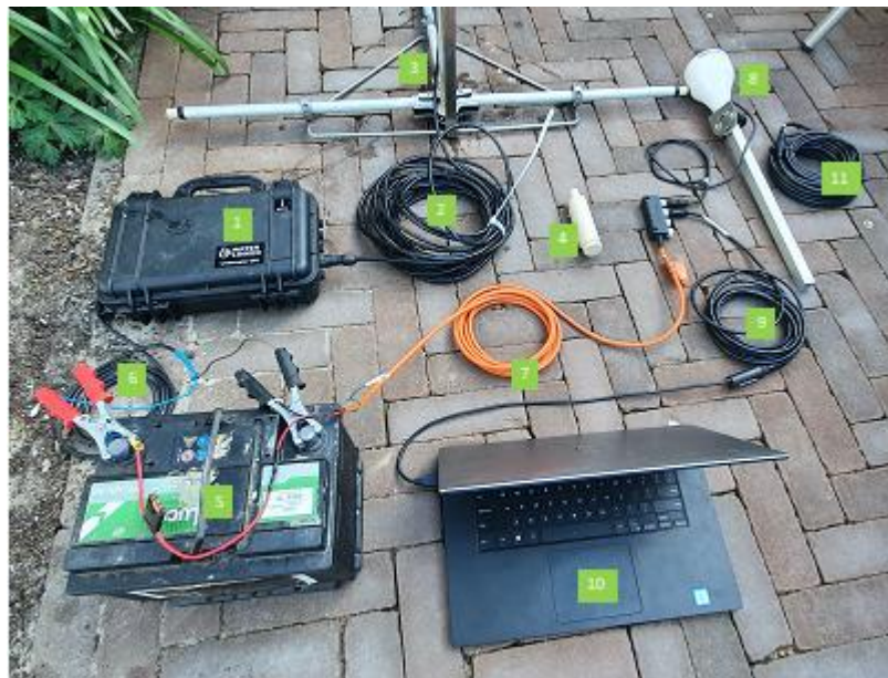
Figure 3.9. Overview of parts of the underwater GPS system.
