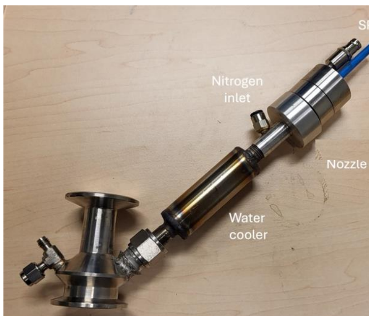
Figure 6. Picture of the adapter and water cooling segment fabricated at RUG to attach the nozzle to a heated reactor.
