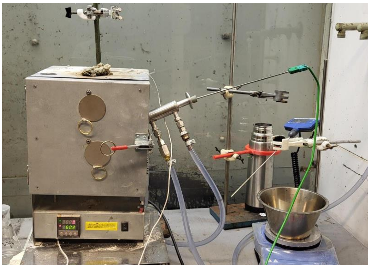
Figure 7: Picture of the test setup used to measure the temperature of the nozzle when connected to a reactor at 600° C.
