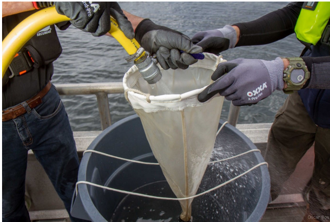
Figure 24. Sampling of oyster larvae by filtering seawater from above the seafloor.
