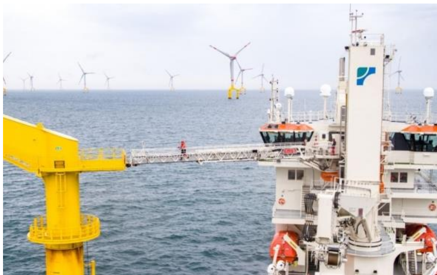
Figure 3-1: Picture of the SMST gangway to transfer from the Acta Auriga to the wind turbine
