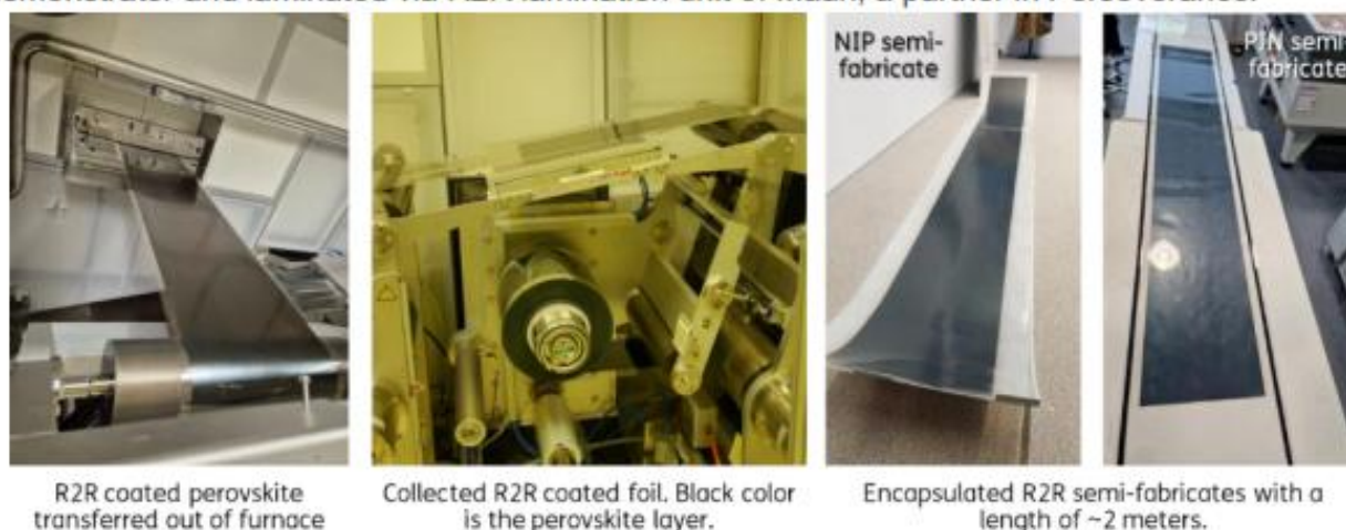
Figure A: Demonstration of the output of D1.1. R2R coated perovskite semi-fabricates were encapsulated. These semi-fabricates were in NIP and PIN architecture and the processed material has been used to make functional devices, and screen encapsulants in other work packages.
