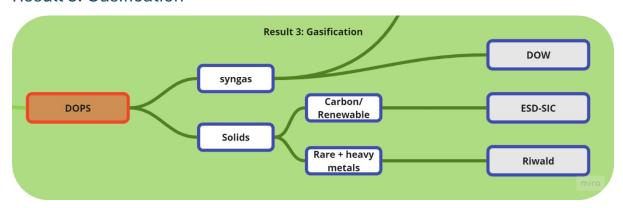
In result 3 waste streams are converted into valuable building blocks (syngas and solid residue) using DOPS proprietary gasification technology "Direct Carbon Immobilisation" to strip hydrocarbons from waste material. Used waste streams include hydrocarbon rich waste such as WEEE, plastics and biomass, also dried paper sludge and screening rejects from the paper industry.
