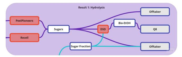
In result 1 waste streams are converted into valuable building blocks using hydrolysis. These waste streams at least include agricultural waste, wet and waterproof paper streams, primary & secondary sludges, and complex and voluminous biomass streams. Recell, PeelPioneers, and DSD are the technology providers in this workstream.
