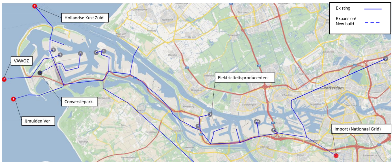
Figure 18: Network topology for electricity in the Port of Rotterdam regional model.
