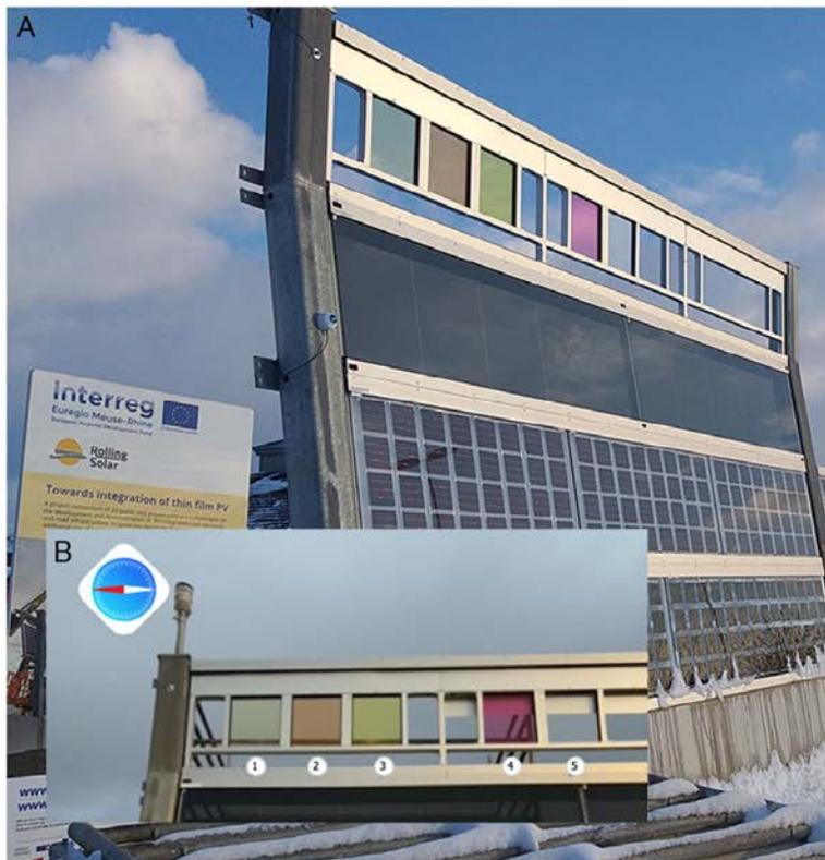
*Figure 17. A) Test setup in Rosmalen, The Netherlands, the tinted rectangles at the top of the structure are the LSCs described in this report. B) The orientation of the LSC support structure, the numbers correspond to the following luminophores: 1) InP, 2) CuInS<sub>2</sub>, 3) CdSe, 4) Lumogen, 5) Blank. The red arrow of the compass at the top left of the picture points toward the geographical North.*
