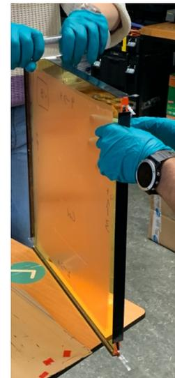
Figure 4. Photograph of LSC with CdSe/ZnS NCs, during the attachment of solar cell strips at UU.
