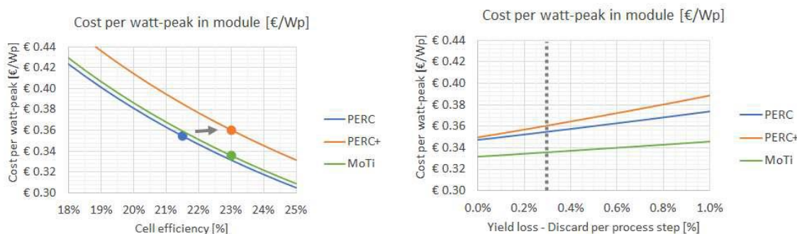
Figure 1: Cost estimates from the RADAR project. Absolute numbers may vary for specific locations, but the largest differences between the trends are related to the number of tools required for the process, which is 6 for MoTi cells and 11-15 for PERC(+) cells. This is reflected in the overall yield loss, the cost of ownership (CoO) and in the floorspace and depreciation costs and are expected to scale with local pricing, due to which the relative differences will remain. Left: Estimates of cost per Wp for bifacial PERC (uniform emitter) and PERC+ (selective emitter) and bifacial MoTi cell as a function of solar cell efficiency. The arrow indicates the efficiency range in which a transition from a simple to a more complex solar cell process is required. Right: Dependence of cost/Wp on yield loss for assumed efficiencies of 21.5%, 23% and 23%, respectively (indicated by dots in the right graph).
