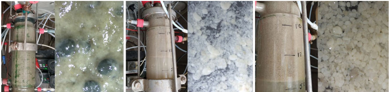
Figure 1. – Granulation process of VFA producing biomass (white-yellow color) over time.
