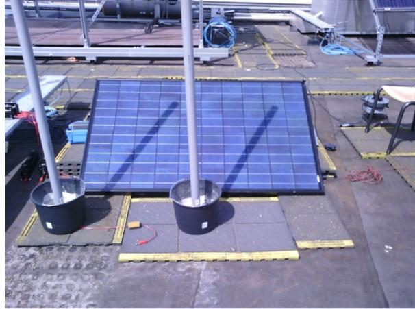
Figure 8: Pole shadow testing setup.
