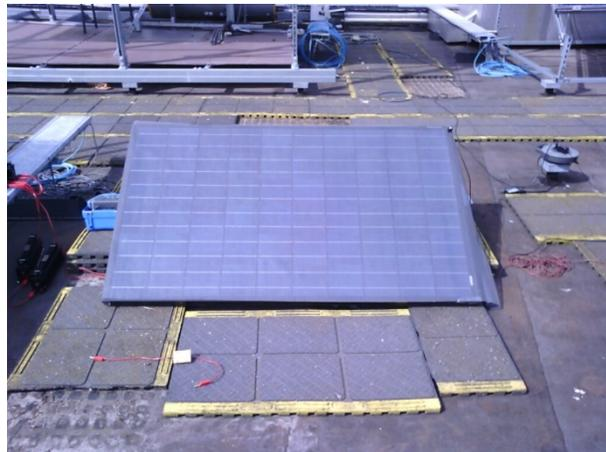
Figure 10: Homogenous fouling testing setup.
