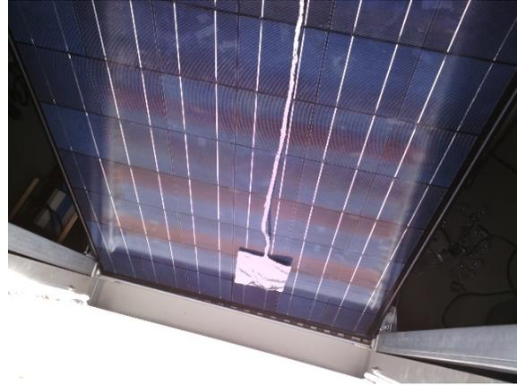
Figure 13. Example of the object for creation of shadow on the PV panel. In the figure it is hanging on against the panel during one of the test rounds
