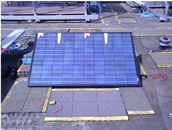
Figure 9: Bird drop testing setup.
