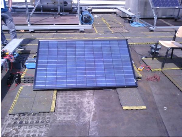
Figure 7: No shade testing setup.
