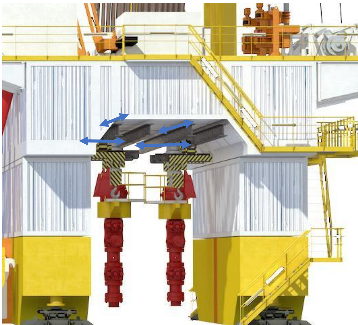
Figure 20: BOP handling system for two BOPs
