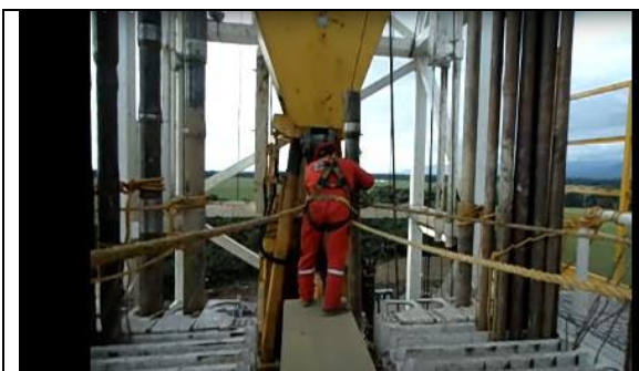
Figure 5: Conventional pipe tripping: 1 person at 25 meter height handler pipe from the setback towards well centre
