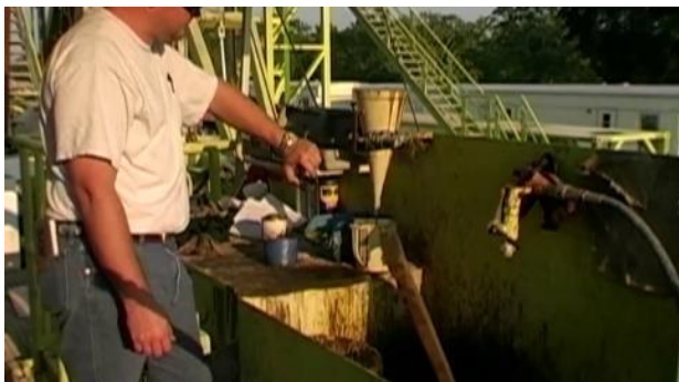
Figure 15: Conventional mud property testing with funnel and watch
