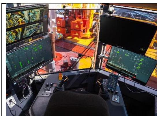
Figure 2: Integrated Huisman drilling parameter control
