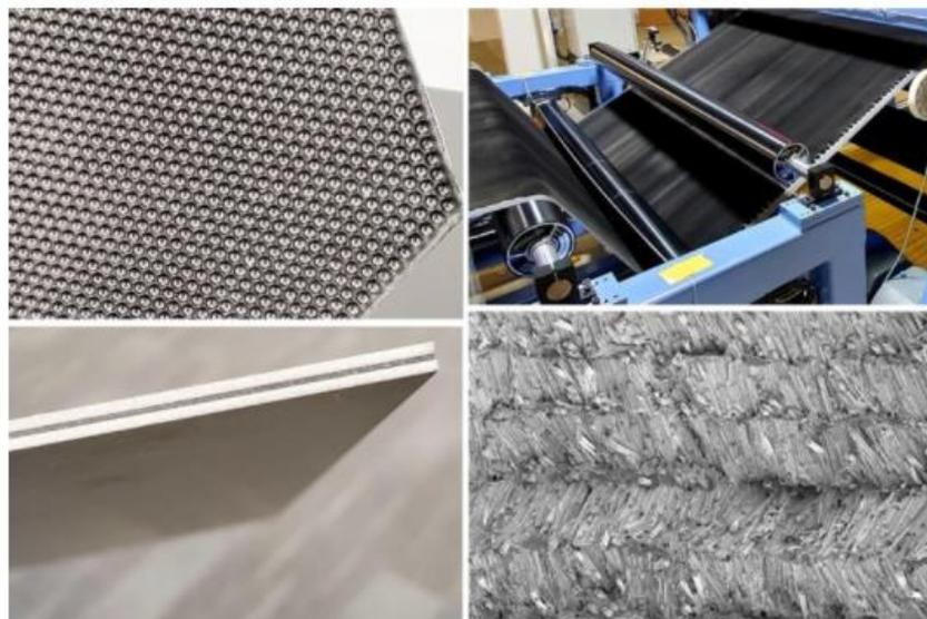
Figure 16 - The manufacturing process of ZRT films (top right) based on z-direction oriented carbon pitch-fibers (bottom right) and use of the material in sandwich sheet and micro-dimple thermoformed plate for non-metallic heat exchanger (top left). [55]
