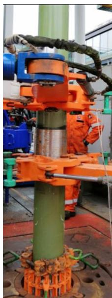
Figure 11 - Running of a composite tube (source: Huisman HCT Brochure).
