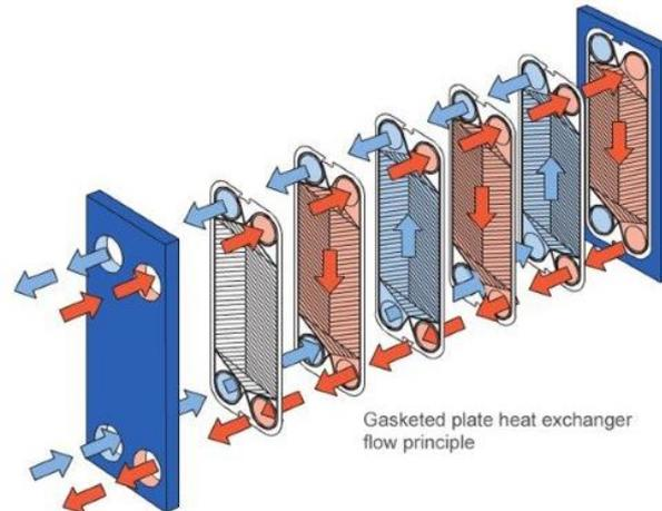
Figure 15 - Working principle of a plate heat exchanger. [50]
