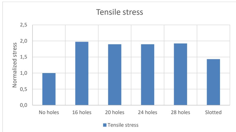
Figure 8 – Normalized stress concentrations at the hole / slots.
