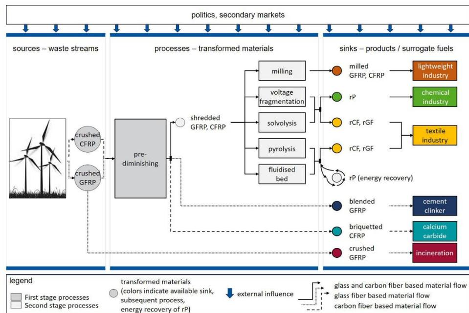
Figure 17 - Recycling and recovery options for GFRP and CFRP for wind turbine rotor blades. [52]
