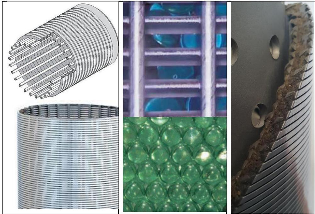
Figure 2 Various well screen lay-outs. Left: wire wrapped screen, middle: prepacked glass beads, right: prepacked gravel (source: www.hpwellscreen.com).
