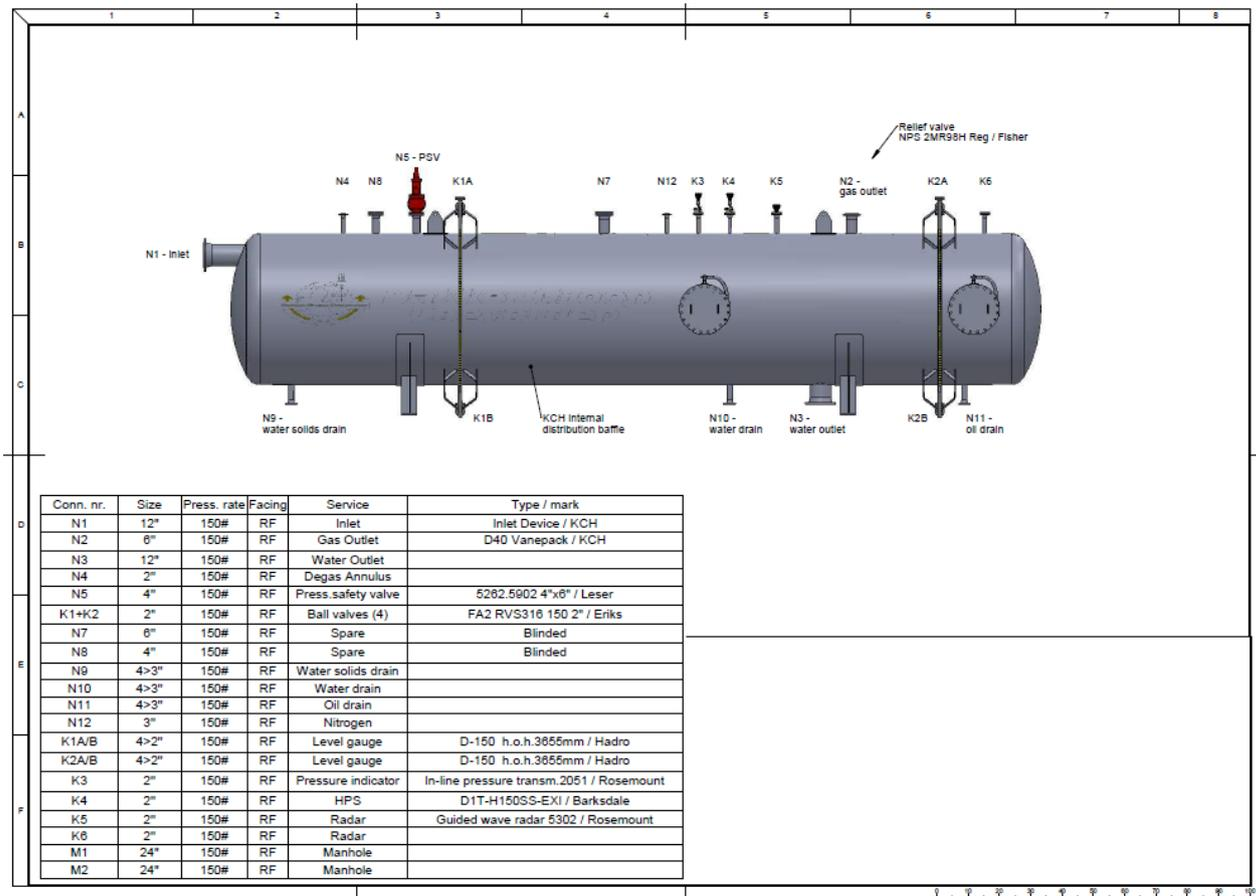
Figure 13 - Schematical picture of the separator and its connections.
