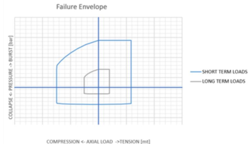
Figure 10 - An example of a load bearing envelope plot for composite casing for both short and long term loads. Source: Huisman
