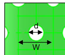
For the analysis, a representative material has been chosen, based on the material properties from Figure 6. This assumes a unidirectional lay-up, which is stacked in a 0, 0, 90 lay-up. In other words, two thirds of the fibres are in axial direction, one thirds in circumferential. Each ply is assumed to be 0.00125mm thick. This pattern is repeated over the entire thickness. The model is created out of shell elements, using the composite lay-up functionality in Abaqus.
