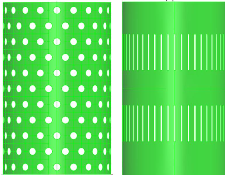
Figure 5 – (Left) Perforated pipe with 16 holes at a 60° pattern and (right) slotted pipe design.
