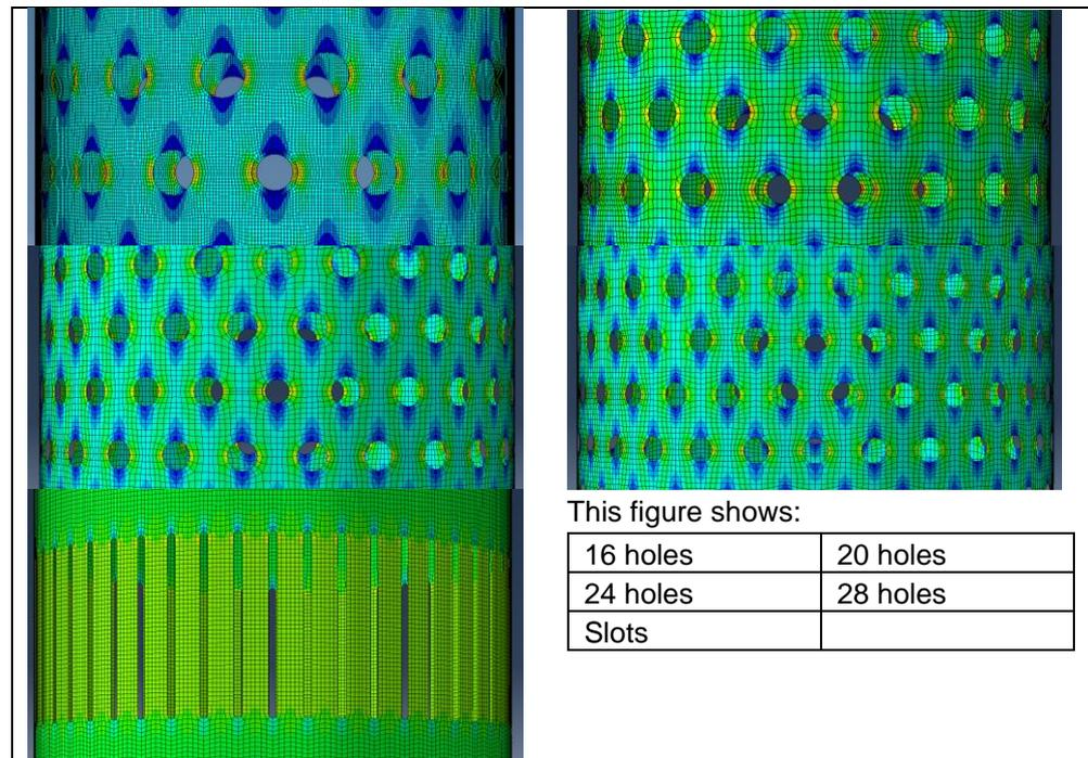
Figure 7 – Overview of stress distributions in the slotted pipe.
