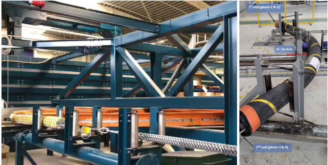
Figure 3.7 (left) Tensile bending test on a 3-core power cable with integrated FO-sensing unit. The sheave wheel diameter is 6 meters. (right) 3-point bend testing on another 3-core power cable with integrated FO-sensing unit.
