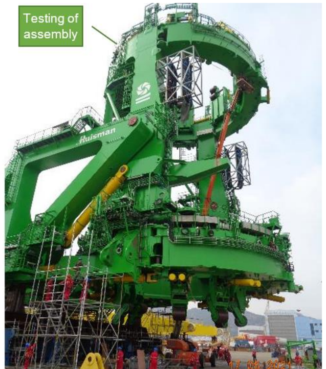
Figure 6-7: Huisman China: Fabrication, assembly and testing of the Y-skid, gripper frame
