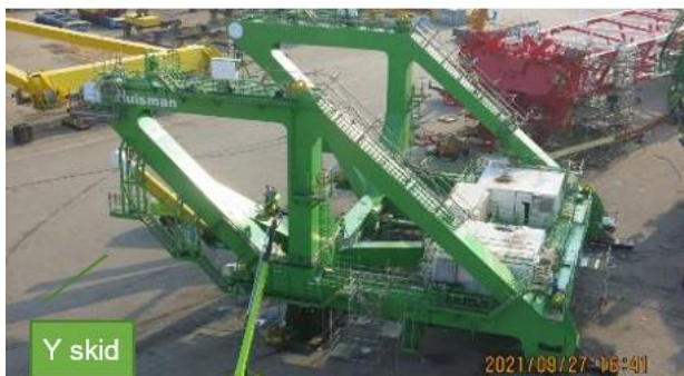
Figure 6-7: Huisman China: Fabrication, assembly and testing of the Y-skid, gripper frame
