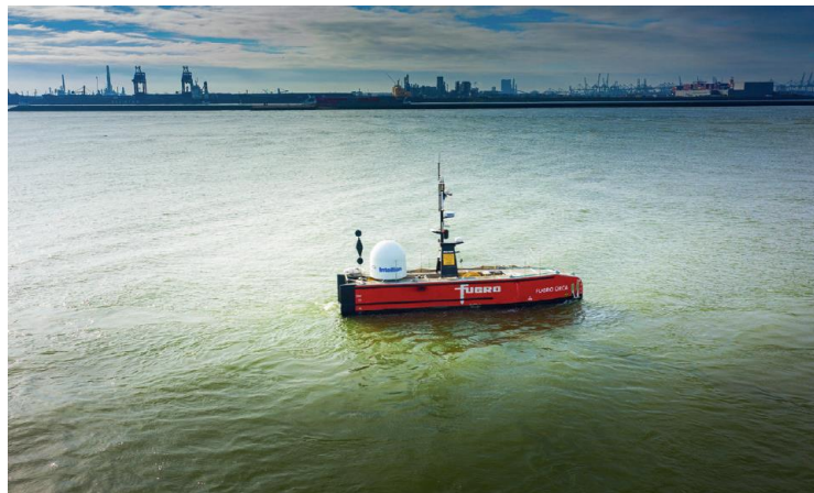
Figure 1: “Fugro’s USV-ROV out of the Port of Rotterdam for its first commercial project”
