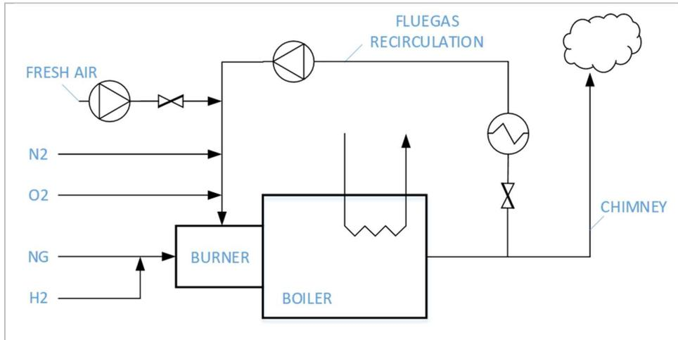
**Figure 4.10: System configuration diagram of oxyfuel test installation**
