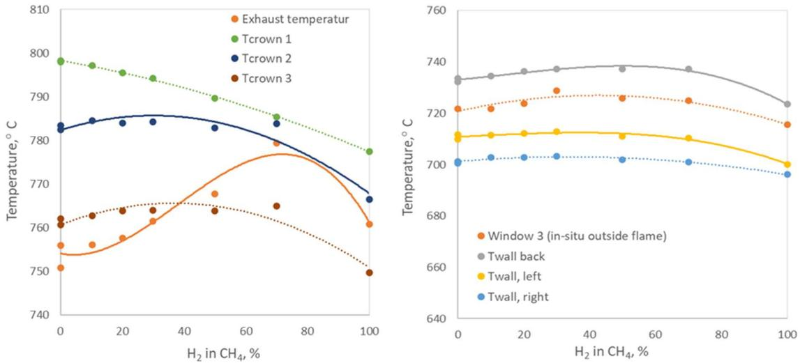
**Figure 4.14** Left: in-situ temperature measurements in window 2 (including flame) and window 3 (outside flame). Right: thermocouple measurements at different positions near the walls.
