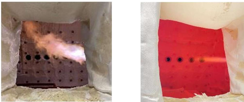
**Figure 4.7: H<sub>2</sub>/O<sub>2</sub> flame using a natural gas oxyfuel burner (left) and a H<sub>2</sub>/air flame using a high velocity burner (right)**
