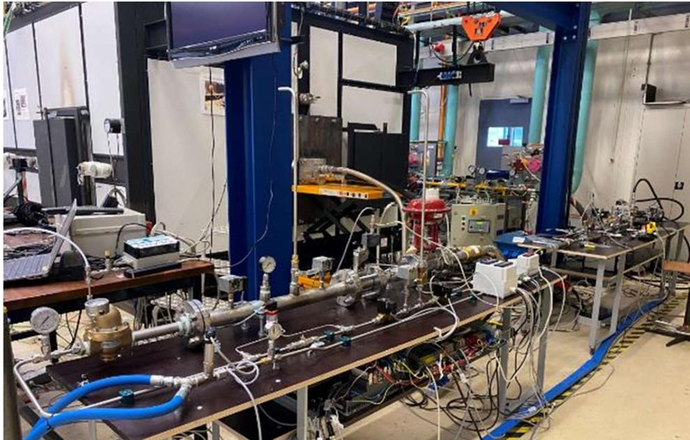
*Figure 3.4: DNV's test facility including 500 kW high temperature kiln equipped with oxyfuel supply system(in front)*
