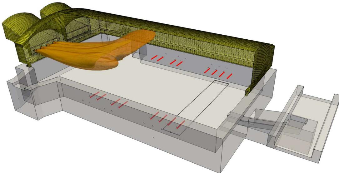
**Figure 6.2: Schematic view of the regenerative end-port container glass furnace for which the impact of combustion air preheating temperature on NO<sub>x</sub> emissions in case of hydrogen combusted is studied**
