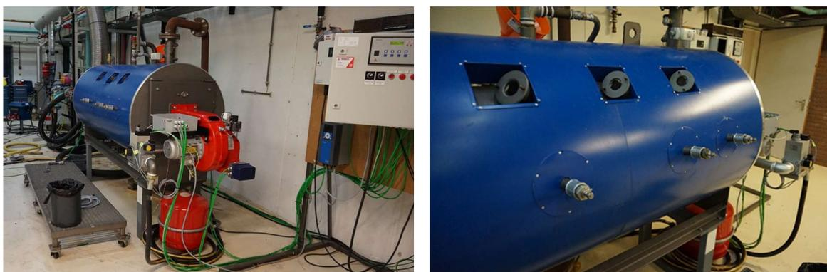
**Figure 3.1 : 450 kW boiler and forced draught burner. The boiler has three quartz windows for flame structure observation.**
