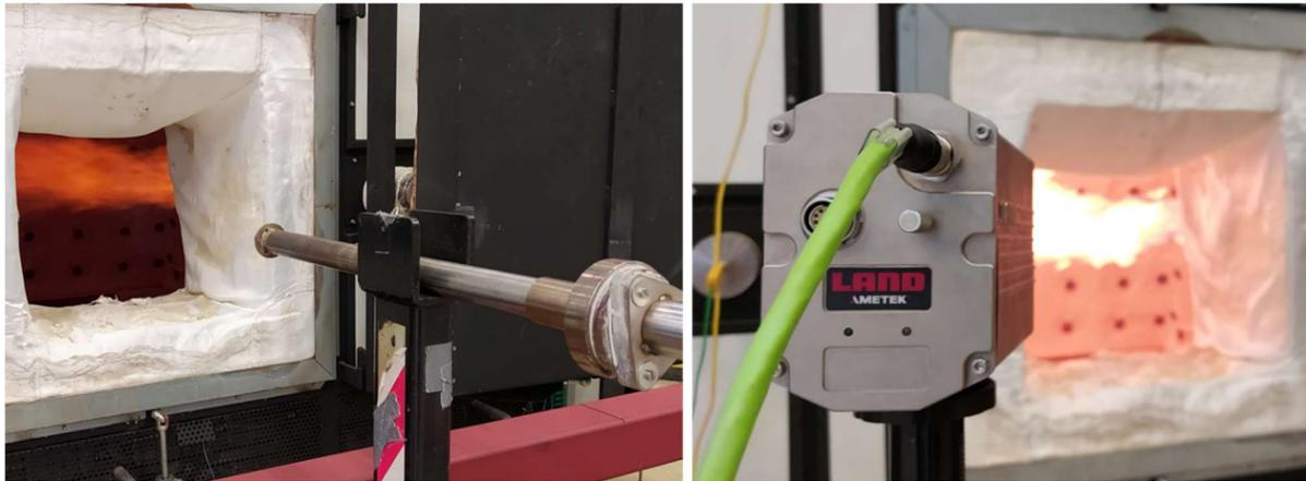
Figure 5.1 Measurement techniques used during burner test program: radiation flux sensor (left) and IR camera (right)
