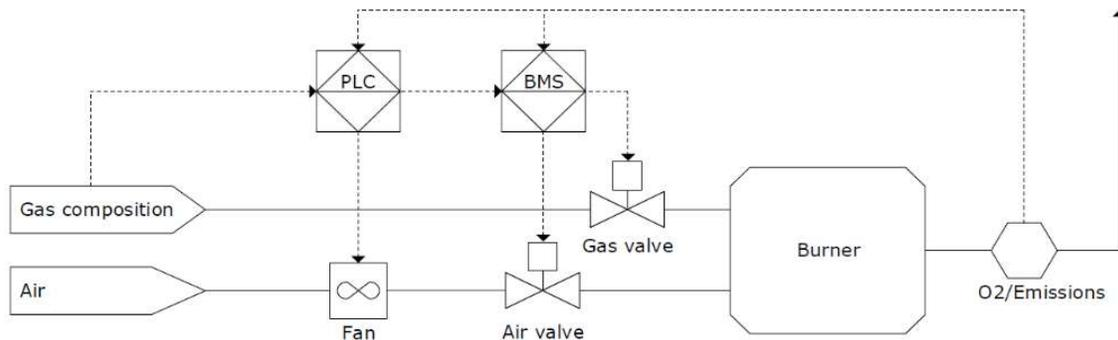
**Figure 3.5: Schematic of the burner setup including fuel-adaptive control system**
