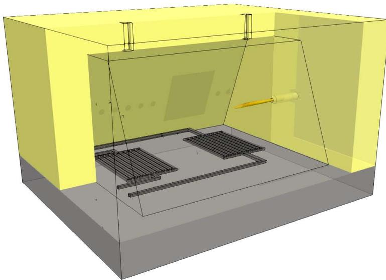
**Figure 6.1: Geometry of the pilot combustion furnace that is simulated with the CelSian CFD code GMT-X**
