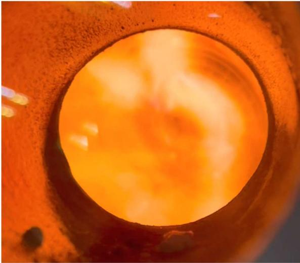
**Figure 4.13: Flame image taken during oxyfuel operation mode**
