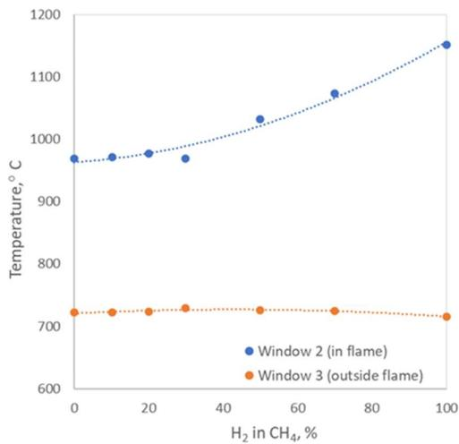
**Figure 4.6: in-situ temperature measurements in window 2 (including flame) and window 3 (outside flame) for burner no. 5**
