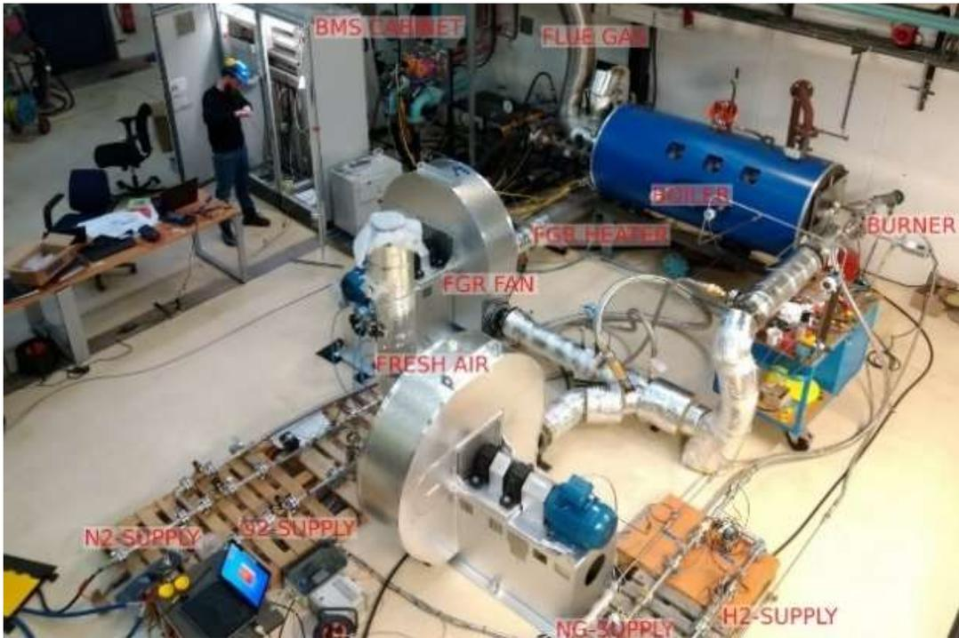
Figure 4.11: Overview of constructed oxyfuel test installation
