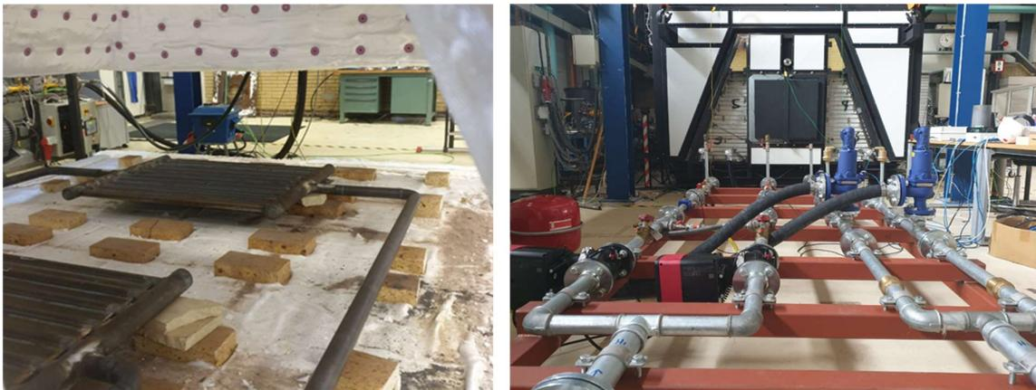
**Figure 3.3: DNV's dedicated test facility including 500 kW high temperature kiln equipped with cooling infrastructure (right) and cooling floors (left) supporting the high temperature experiments**
