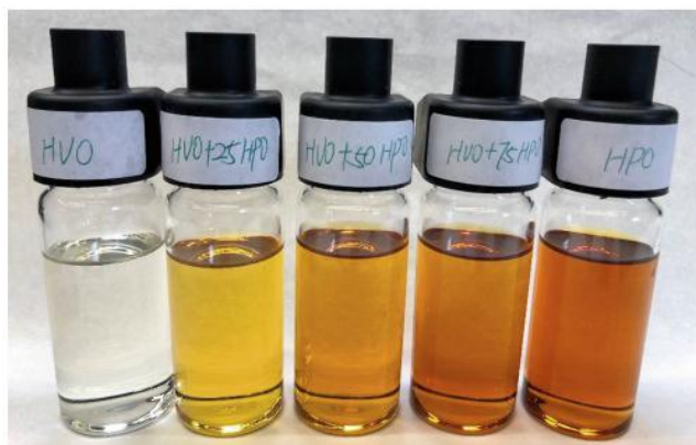
Fig. 3. HVO/HPO fuel blends samples from 0 to 100 vol% blend ratio.
