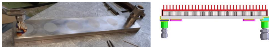
Figure 3.5 TEG panel #4, flue gas heat source, water cooling
