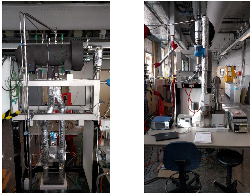
Figure 3.6 Lab setup for testing TEG panel #2
