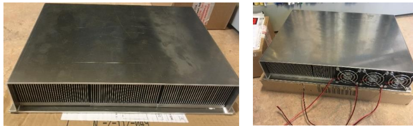
Figure 3.4 TEG panel #3, radiation heat source, air cooling
