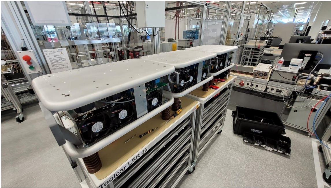
Figure 17 Assembly of the AC/DC and DC/DC stage at Prodrive
