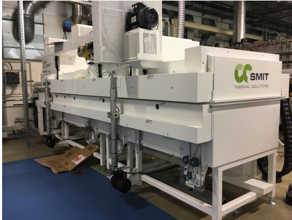
Figure 1 Pictures of the dry and anneal tool for sheet-to-sheet produced perovskite layers developed and built by Smit Thermal Solutions and located at TNO/Solliance.
