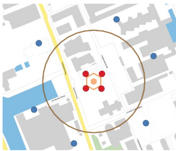
Figure 16. Sketch of possible HT-ATES system for the Ommelanden formation (10 total wells) locations in immediate area of DAPwell. Red and blue dots are hot and cold wells, respectively, brown circle is the maximum thermal zone.
