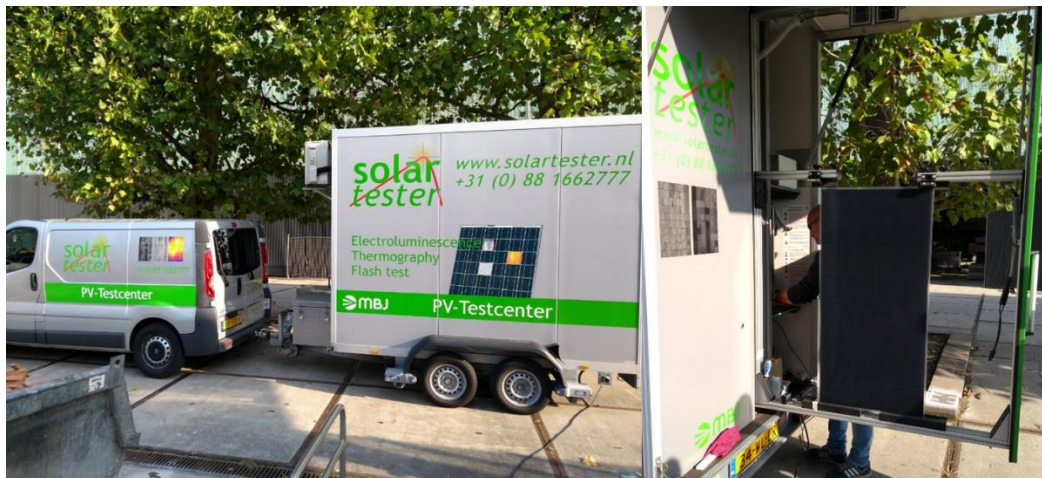
Figure 4: (Left) Mobile PV tester (Right) Placement of a thin film PV module in the tester
