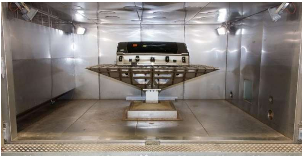
Figure 7 - Thermal & vibration test setup
