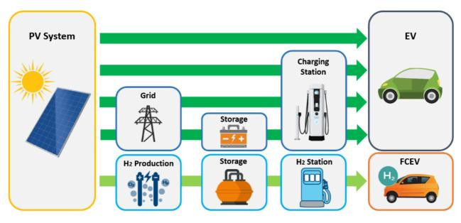
Figure 2. Schematic of options for PV to EV charging.
