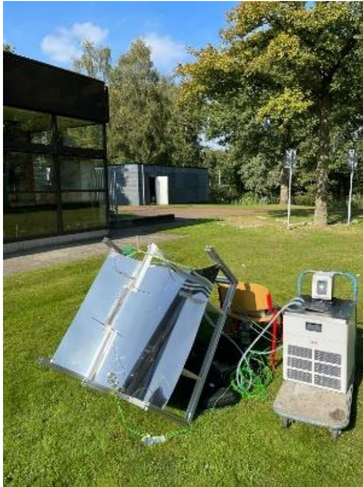
Fig. 15. Experimental setup of the PTC in outdoor experiments.
