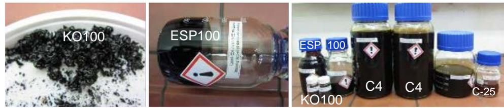
Figure 20 Recovered fractions from the pyrolysis of granulated walnut shells at 500°C
