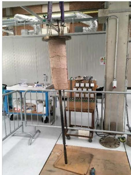
Entrained flow riser reactor insert
