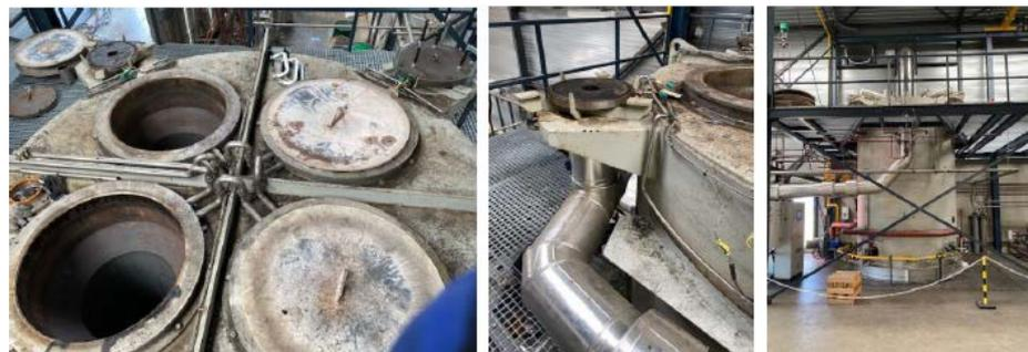
Figure 11 Left, the cylindrical inserts in the RMO furnace, middle the product gas line to the condensers, right, the RMO furnace, front view
