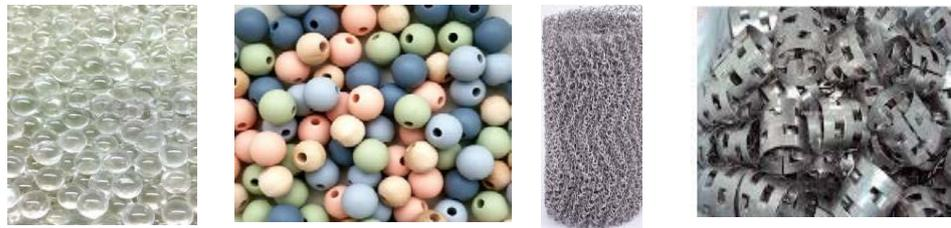
Figure 36 Different materials used for supporting and dispersing viscous pyrolysis oil
