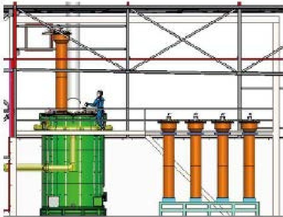
Figure 10 Pilot-scale RMO reactor set-up with in green the natural gas – fired furnace and in orange the biomass filled cartridges.
