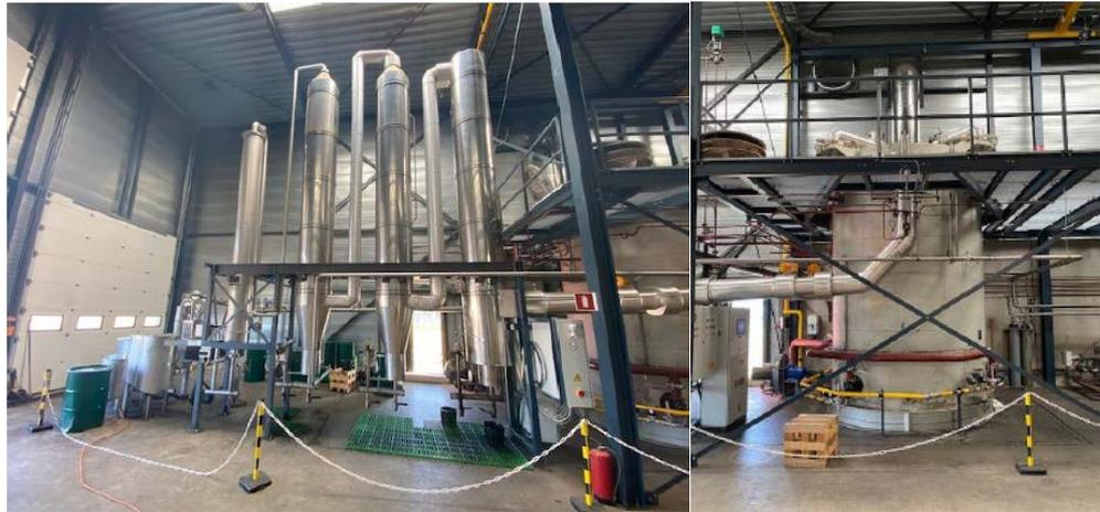
Figure 12 The product gas condensation set-up (left), connected to the RMO (right)
