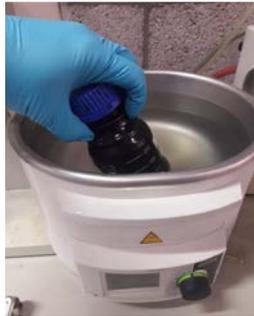
Figure 35 Pyrolyzed oil is warmed up to allow pouring it out of the bottle
