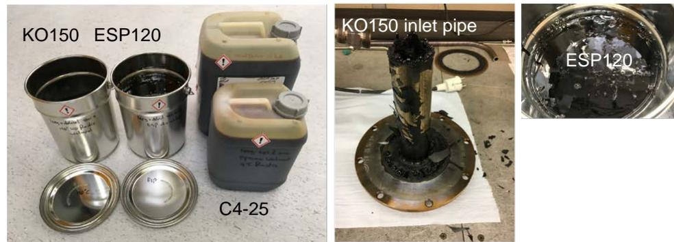
Figure 24 PYRENA pyrolysis oil fractions from granulated walnut shells
