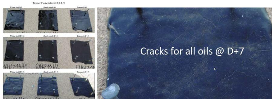
Figure 48 Weatherability tests ESP120 : bitumen blends
