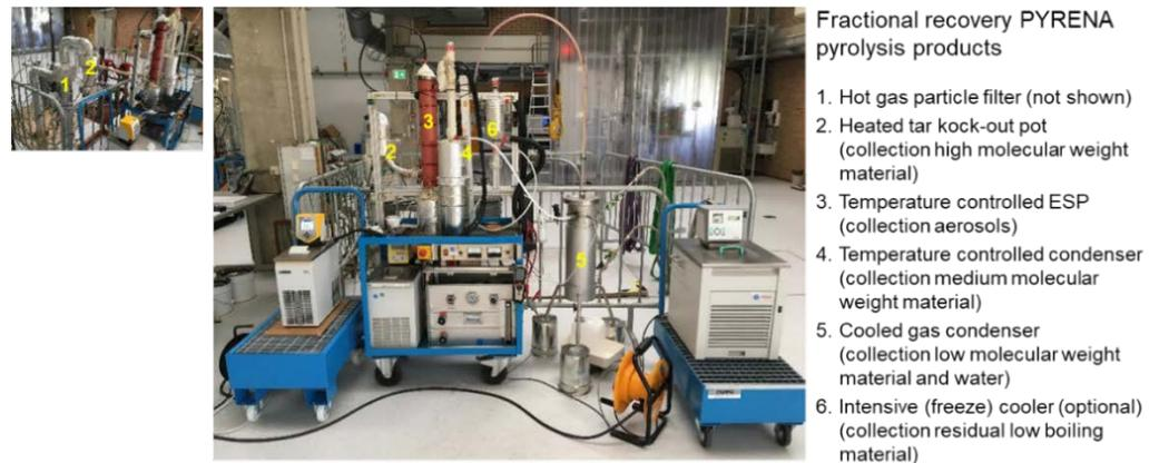
Figure 8 PYPO (PYrolysis Product Obtention) configuration for product recovery
