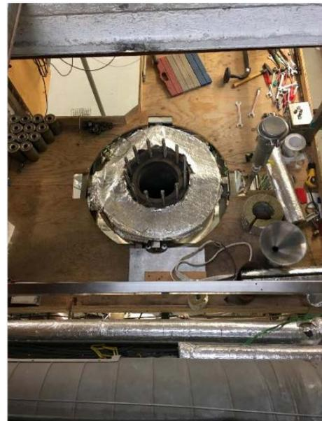
Bubbling fluidized bed char combustion vessel (top view)
