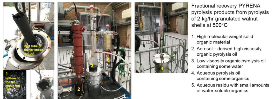
Figure 9 Typical product fractions collected in the PYPO
