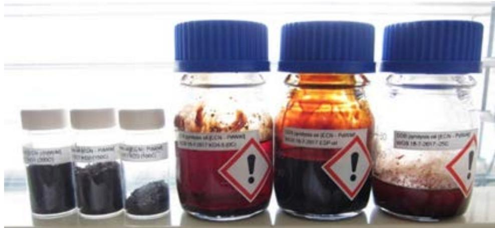
Figure 13 The six collected pyrolysis liquid fractions from the pyrolysis of DDB with (from left to right) the KO200, KO150, KO100, C0, ESP and C-25 fractions
