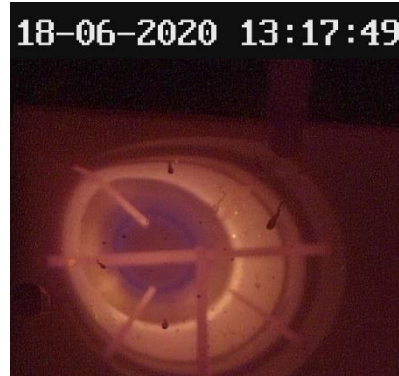
Figure 2 100% hydrogen - baseload conditions
