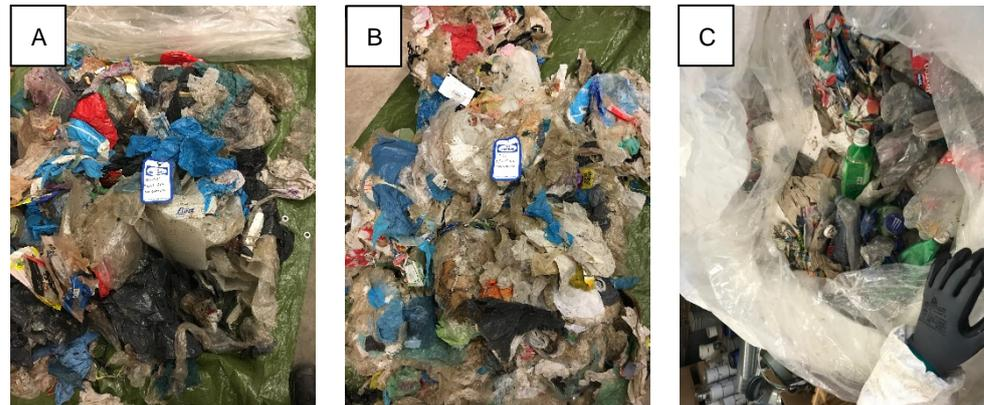
Figure 3.1: The three plastic streams “as received” at TNO: A) DKR310 Small Foils (2D); B) DKR310 Big Foils; C) Mixed Plastics
