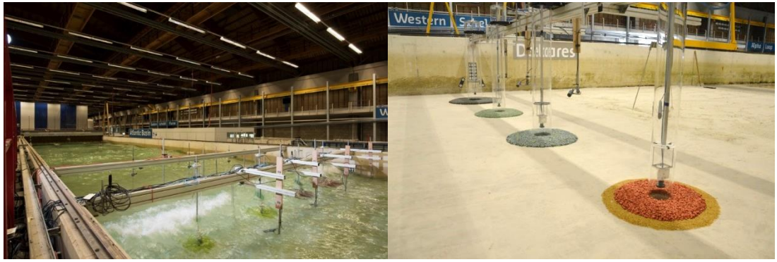
Figure 3.2 Breaking wave during in the test section for loose rock scour protections (left) and four scour protection layouts just before testing.
