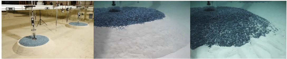
Figure 3.5 Photo and underwater camera images showing the falling apron behaviour around the edge of a protection as a result of bed level lowering in a physical model test setup.
