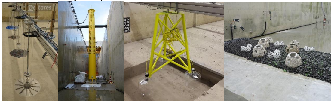
Figure 2.1 Several scale models of different foundation types from left to right: transparent monopile for small scale test, monopile scale model in the Delta Flume, SBJ scale model and cable protection
