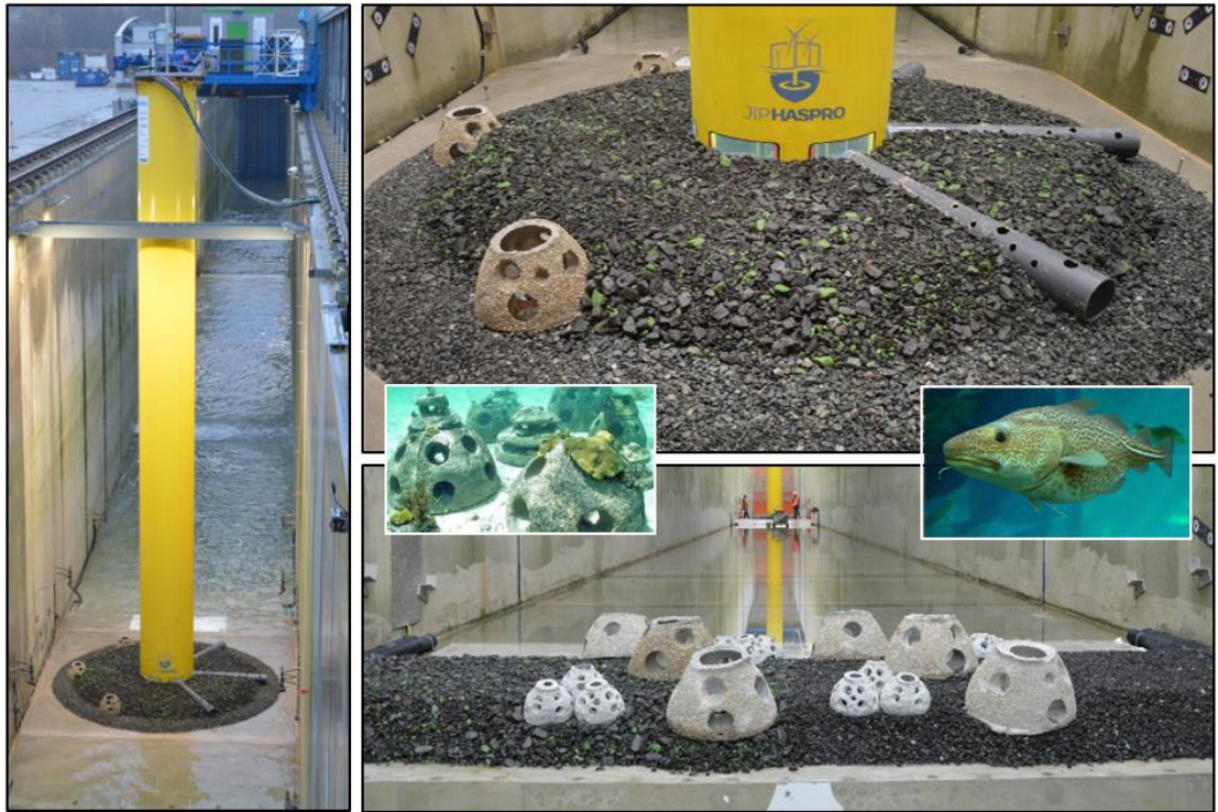
Figure 3.15 Eco-friendly scour protections with various artificial reef elements tested in Delta Flume.
