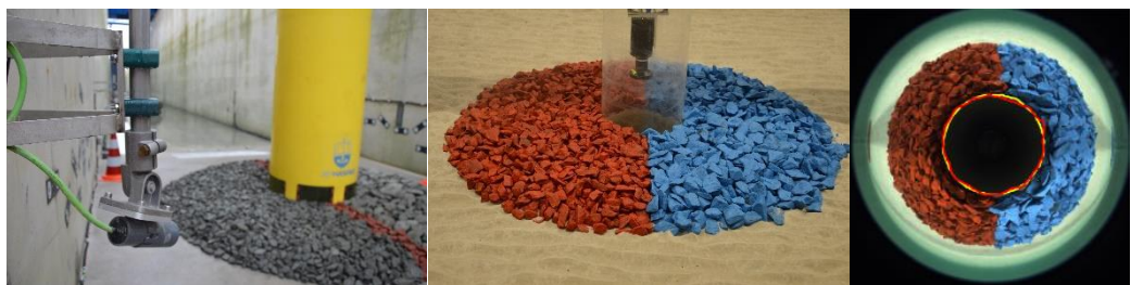
Figure 2.4 Underwater and internal cameras were used in all test programs to record the scour protection behaviour. From left to right: underwater camera in the delta flume, internal camera inside a transparent monopile foundation in the Atlantic basin, with the corresponding view from the camera on the protection. Smart image recognition is done to track the height of the rocks and sand layer at the pile interface.
