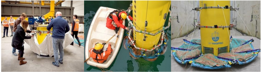
Figure 3.13 First unfolding tests together with the JIP participants (left), accessing the flume with a boat to re-attach the scour protection (middle) and unfolded system in a drained flume (right).
