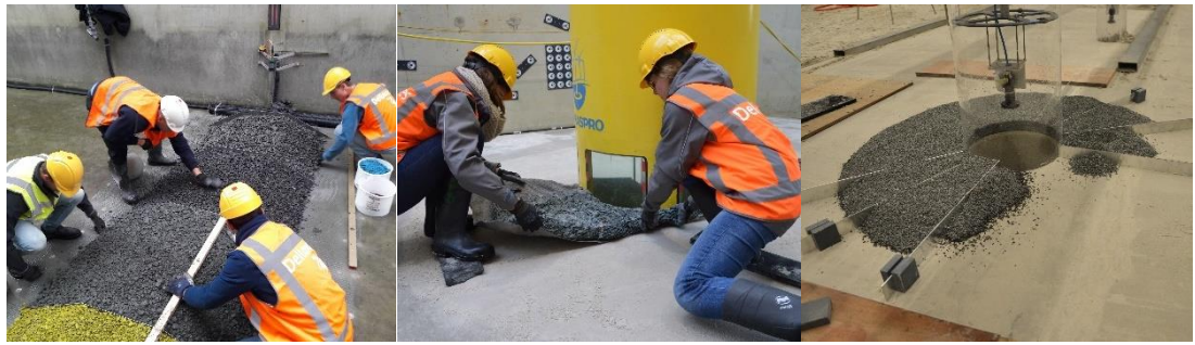
Figure 2.2 Example of scour protection from left to right: installation of a rock berm, placement of gabions around the monopile in the Delta Flume and installation of a scaled loose rock scour protection in the Atlantic Basin.
