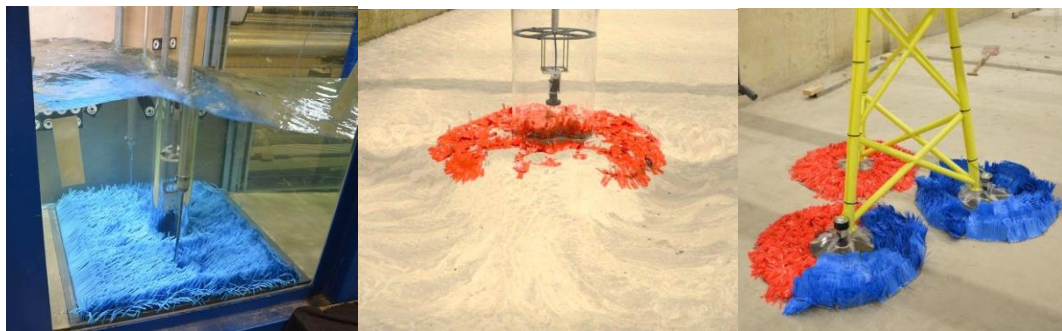
Figure 3.7 Artificial vegetation scour protection tested at a monopile in the Scheldt Flume (left), at a monopile in the Atlantic Basin (centre) and at an SBJ in the Atlantic Basin (right).
