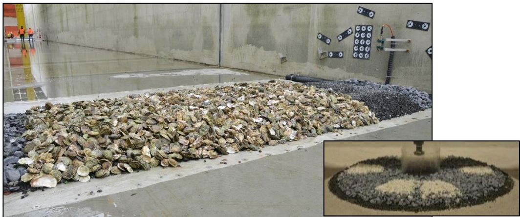
Figure 3.17 Eco-friendly scour protections with loose shell material tested in Delta Flume (fully covering a cable protection) and Atlantic Basin (installed in patches around a monopile) for JIP HaSPro.
