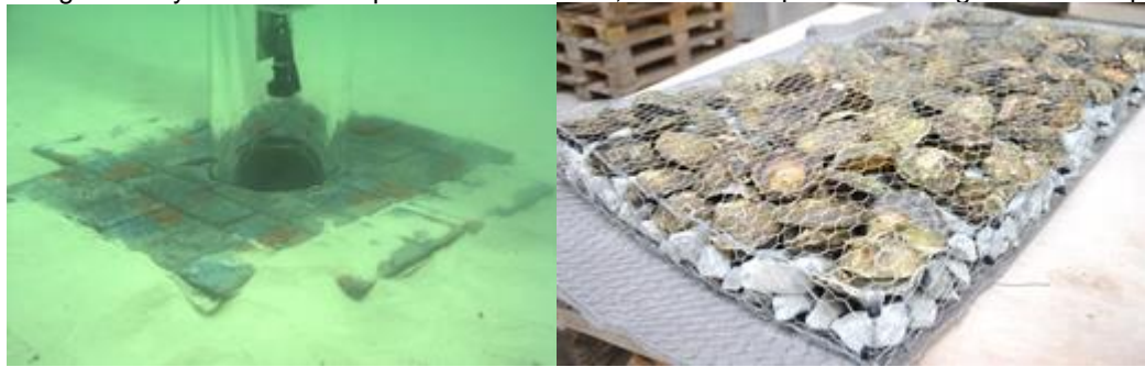
Figure 3.2 Gabion mattresses tested in the Atlantic Basin (left) and a gabion mattress partially filled with oyster shells that was tested in the Delta Flume (right).
