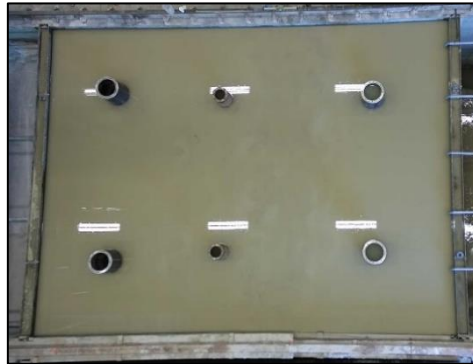
Figure 9: Left: IHC Fundex CP25D pile driver positioned on dragline beams on top of the flume. Right: 6 piles are installed in each soil model.
