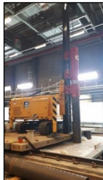
Figure 9: Left: IHC Fundex CP25D pile driver positioned on dragline beams on top of the flume. Right: 6 piles are installed in each soil model.
