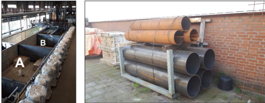
Figure 7: Left: test compartments A and B created for the HyPE-ST project in the Water-Soil Flume. Right: scale 1:20 piles (bottom) and scale 1:30 piles (top).
