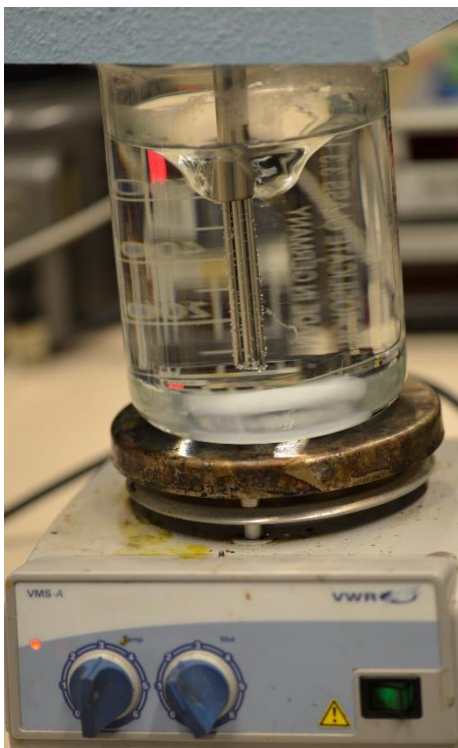
Figure 9: Calibration of PT100's
