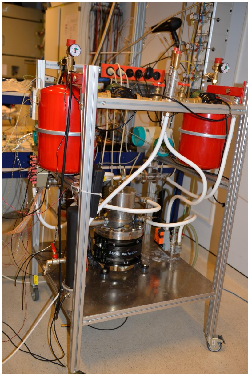
Figure 7: Photo of the test rig showing the heatpump, cooling and heating circuits, flow sensor and buffer vessels with filling ports.
