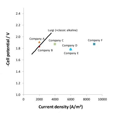
• We see increased current densities while retaining the same efficiency, made possible by cathodes that have been developed for the chlor-alkali industry and improved membranes
