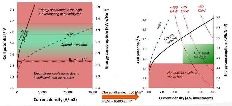
Note: current efficiency is 98% for alkaline and PEM (due to leak currents and gas crossover)
