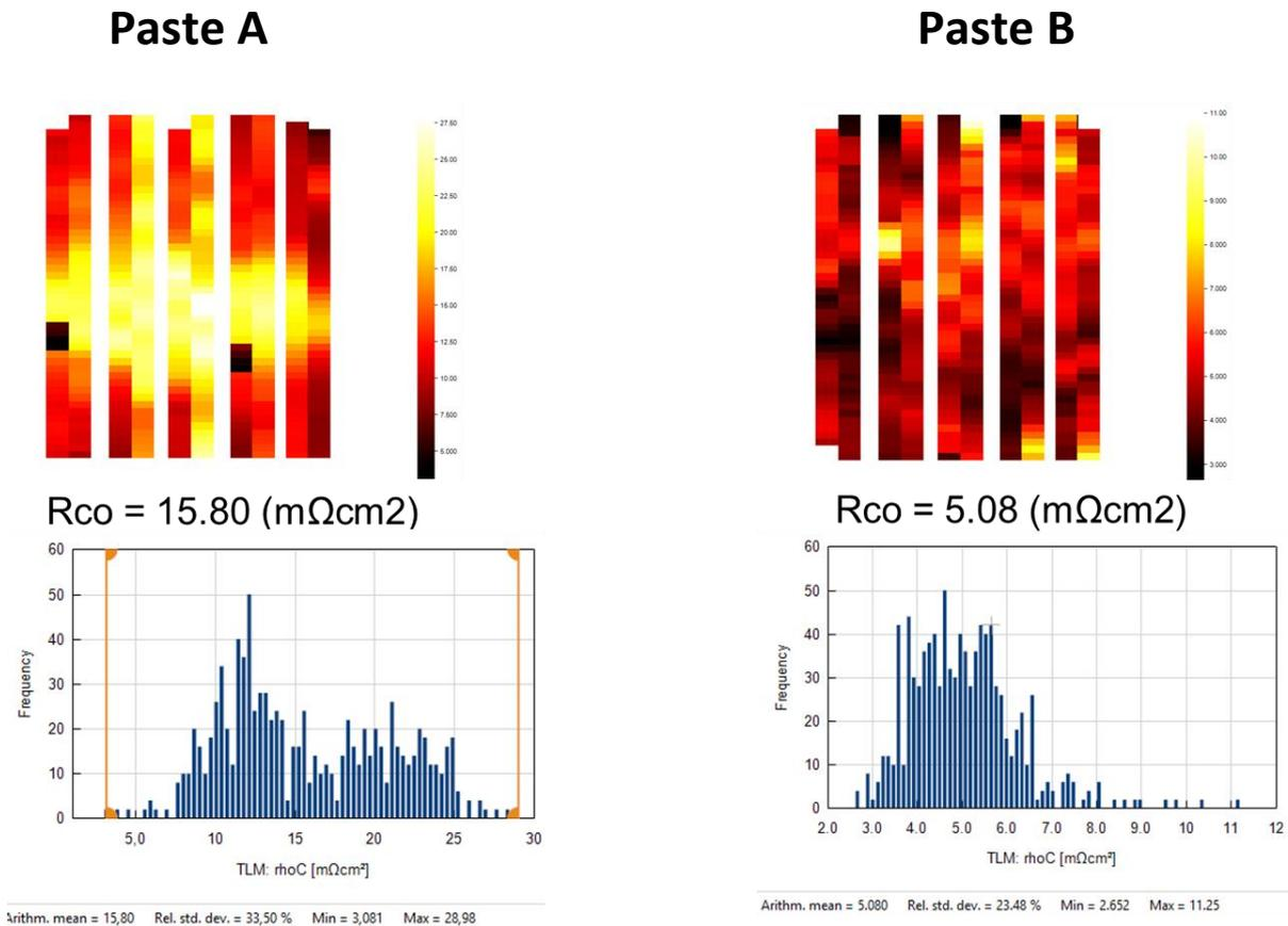
Figure 23. TLM analysis of the contact by Ag/Al pastes on deep Boron emitters (note the different scales in the graphs).
