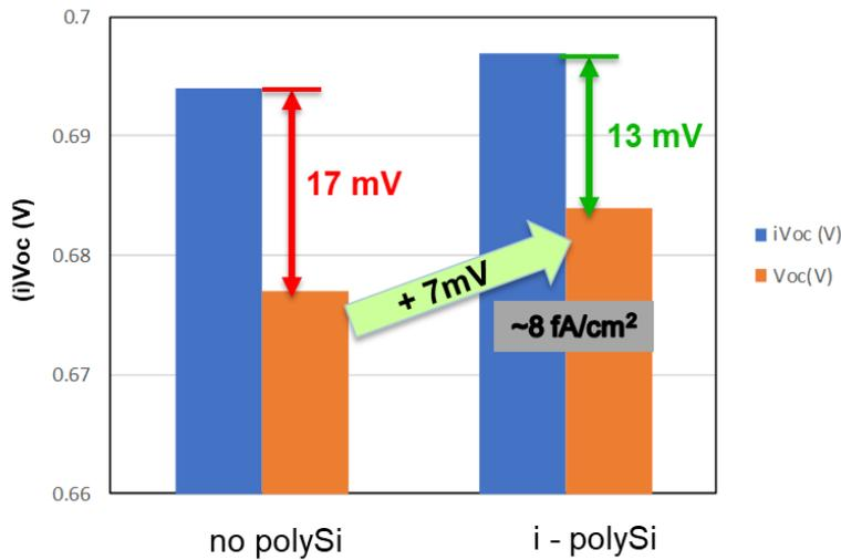
Figure 27. Benefit of the intrinsic polySi layer for implied  $V_{oc}$  (emitter passivation) and  $V_{oc}$  (emitter + contact passivation).
