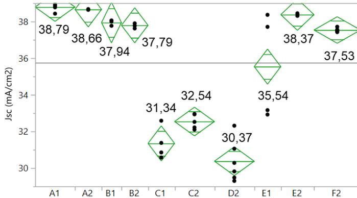
Figure 29. Increase in  $J_{sc}$  due to patterning of the intrinsic polysilicon (splits E1, E2 and F2 compared to C1, C2 and D2).
