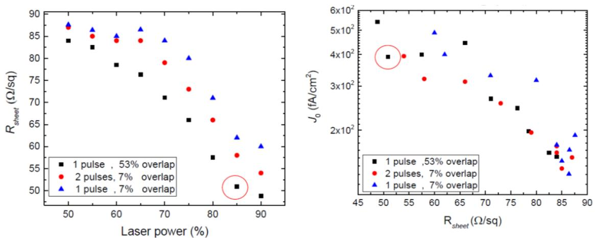
Figure 14.  $R_{sheet}$  of boron doped emitter as a function of laser power and pulse setting (left) and  $J_0$  of the emitter as function of  $R_{sheet}$  (right).
