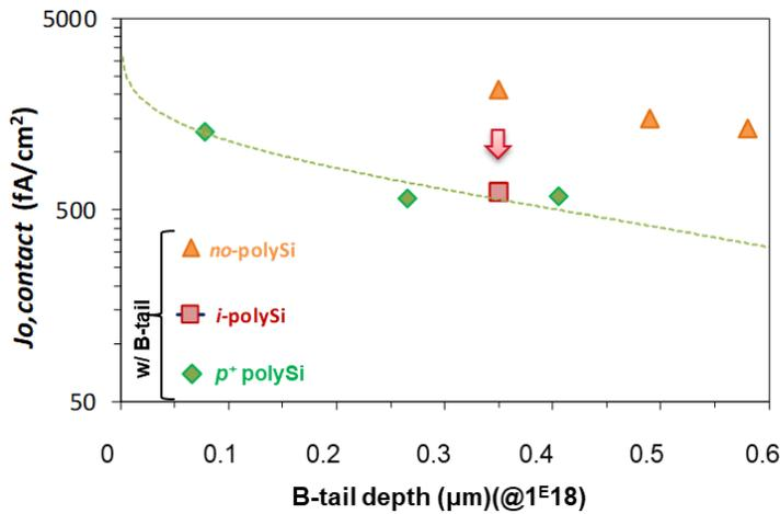
Figure 21. Reduction of  $J_{0,c}$  of emitter contacts by inserting intrinsic polysilicon. The effect is comparable to contacts with p-type polysilicon.
