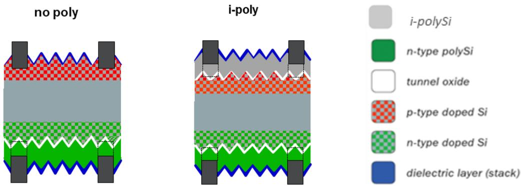
Figure 3. Concept of inserting an intrinsic polysilicon layer under the emitter contacts between emitter and dielectric layer stack.
