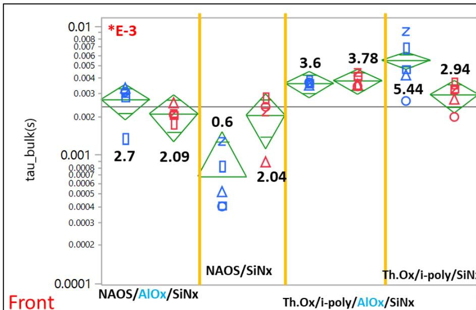
Figure 15. Bulk lifetime exceeding 2 ms for all PERPoly cells, and boosted by the presence of polysilicon to  $\sim >3$  ms.
