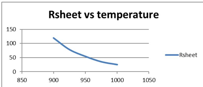
Figure 7. Sheet resistance decreasing as function of diffusion temperature when keeping other parameters constant.
