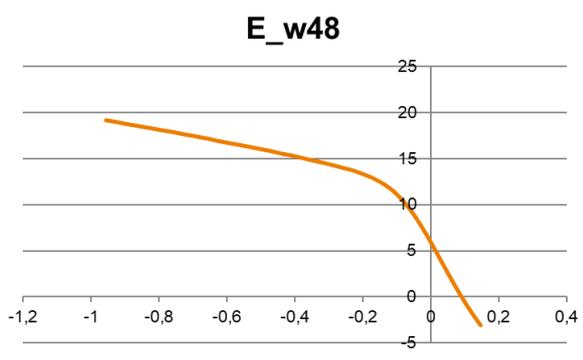
Figure 24. IV curve (bottom), PL image and ECV curves of a solar cell with n-polysilicon/B emitter tunnel junction and Ag contacting the n-polysilicon. Unfortunately the tunnel junction between (n)polysilicon and the B emitter is not effective and leads to a reverse diode resulting in excessive series resistance.
