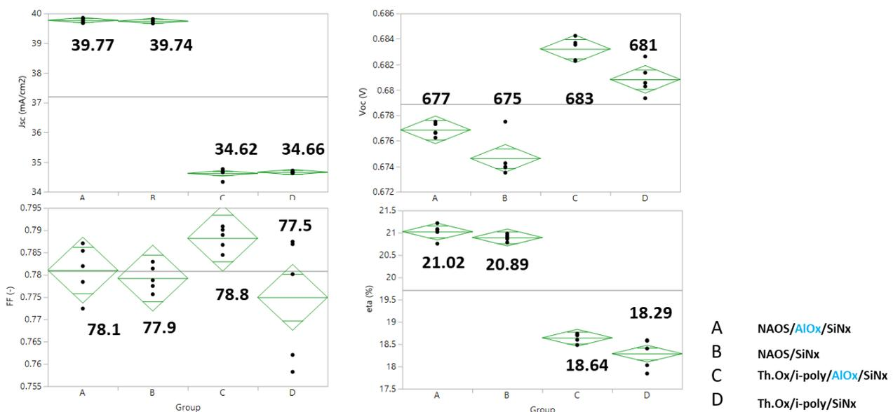
Figure 26. IV parameters of solar cells with two different dielectric passivation stacks, and with and without an additional intrinsic polysilicon layer.
