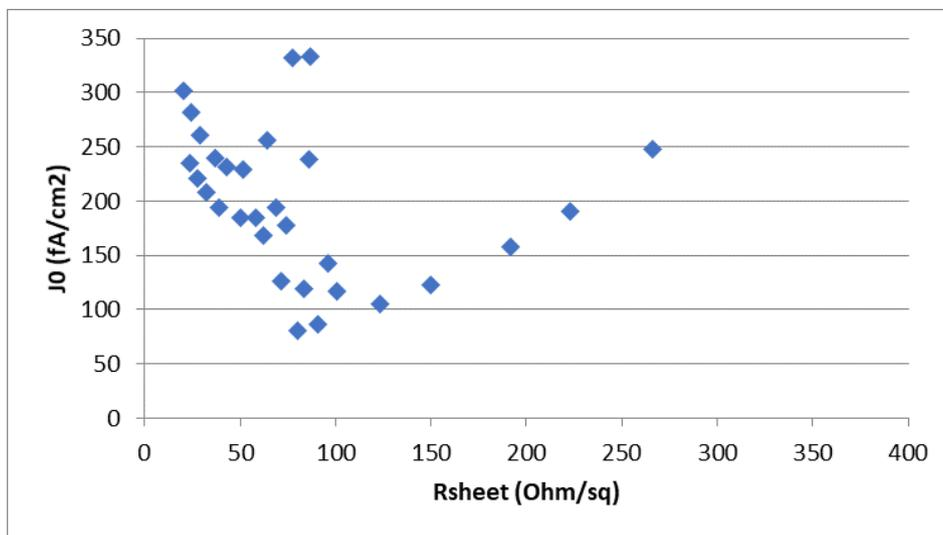
Figure 17. Total  $J_0$  as function of emitter sheet resistance (data shown for 200nm etching depth).
