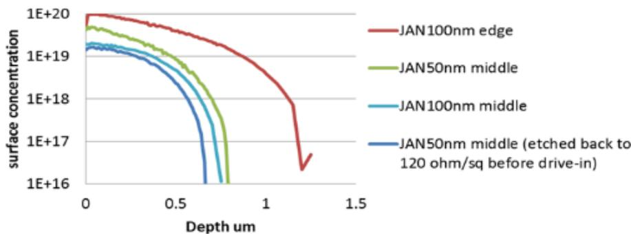
Figure 12. Sherescan (top) and ECV (botto) showing non-uniform doping profile and sheet resistance after long drive in.
