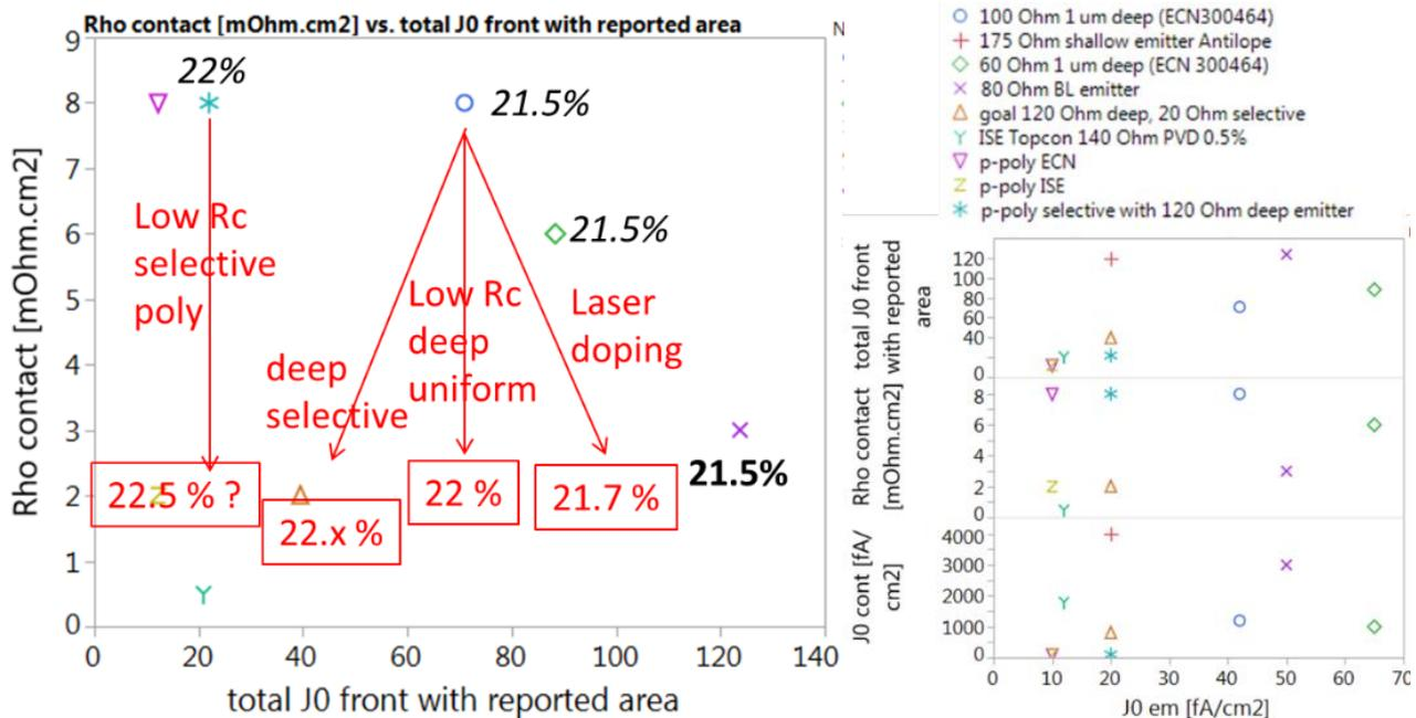
Figure 2. Overview of the different strategies to improve the solar cell efficiency by improving emitter passivation and contacting. The graph on the right shows a summary of different emitters available at the beginning of the project.
