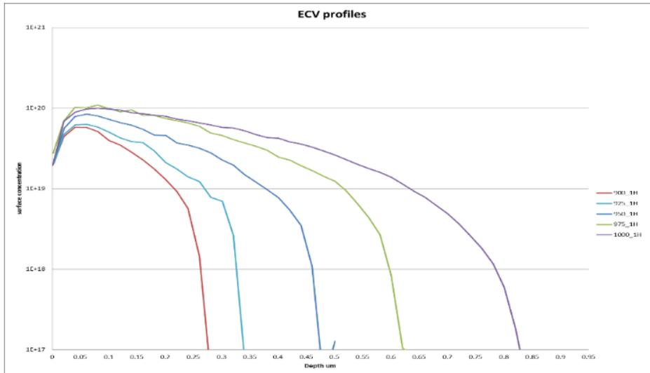
Figure 6. ECV profiles of deep emitters diffused for 1h at temperatures varying from 900°C to 1000°C.
