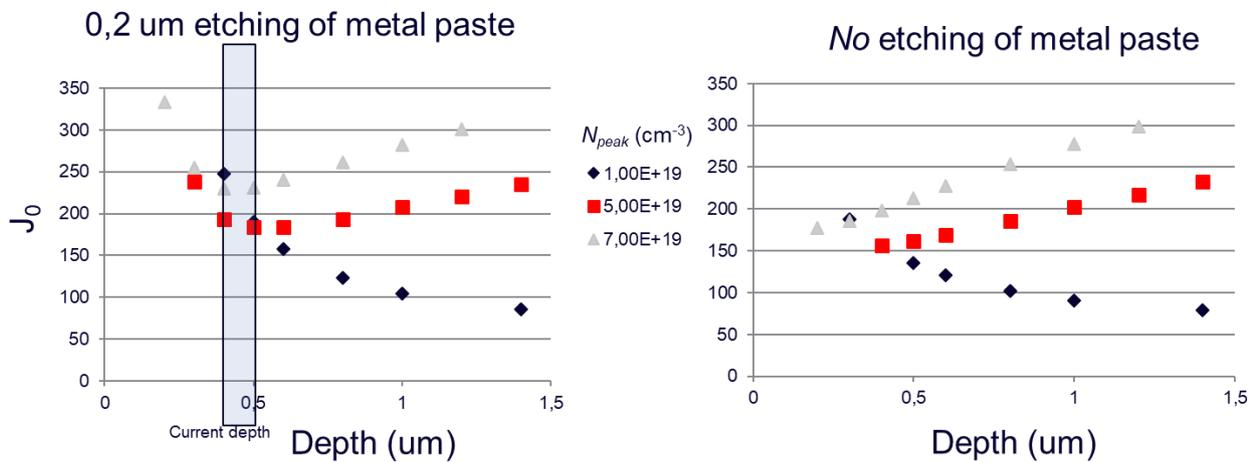
Figure 16. Simulated  $J_{0,contact}$  as function of emitter depth for different peak doping levels. Left: assuming 200 nm penetration of metal paste, right: neglecting penetration of metal paste (ideal non-fire-through contact).
