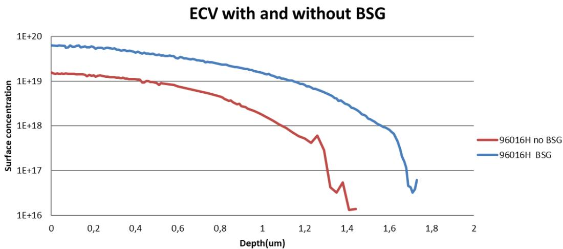
Figure 10. ECV showing emitter profiles for samples where drive-in was done with and without Boron glass (BSG) present.
