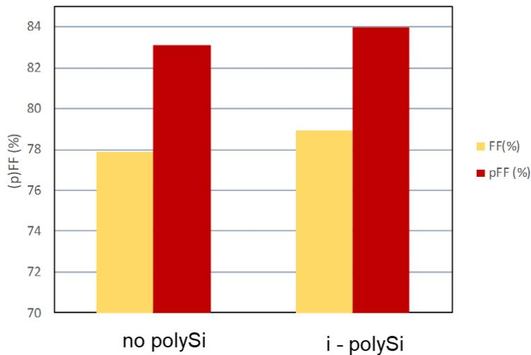
Figure 28. Benefit of the intrinsic polySi layer for the pseudo fill factor (pFF), and resulting gain in fill factor (FF).
