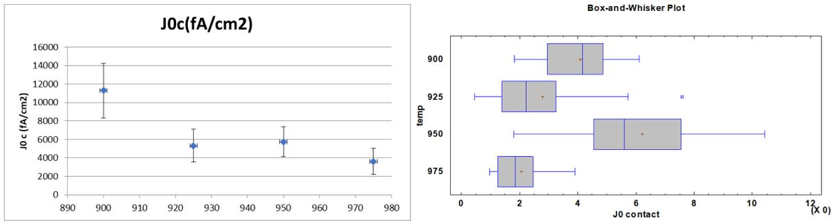
Figure 18. Reduction of contact resistance with deeper and higher doped emitters fabricated with higher drive-in temperature.
