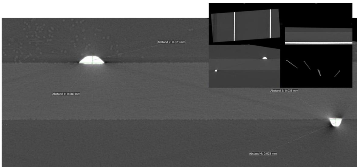
Figure 22. Cross section(s) of a 3-d x-ray scan showing the silicon cell wafer with metal contacts on top and bottom of the solar cell.
