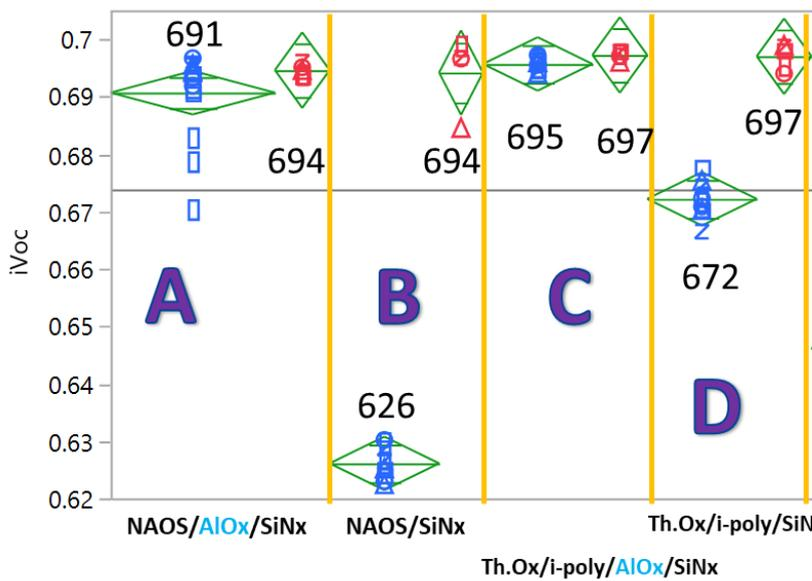
Figure 4. implied Voc before (blue) and after (red) firing for PERPoly half-fabricates with a standard p+ emitter with (A) and without (B) Al<sub>2</sub>O<sub>3</sub> passivation below the SiNx, and a p+ emitter passivated by intrinsic polysilicon and capped with (C) and without (D) Al<sub>2</sub>O<sub>3</sub> layer below the SiNx.
