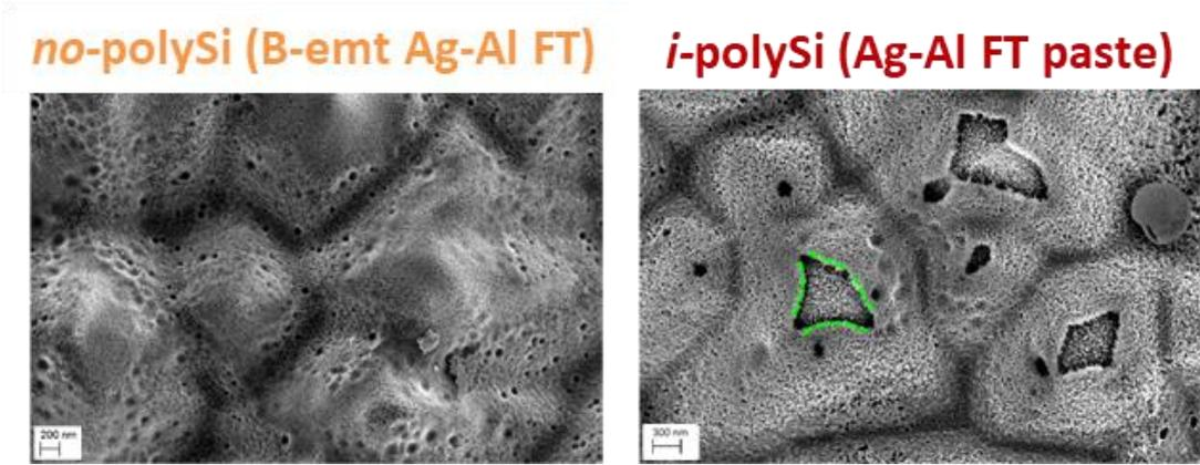
Figure 20. Damaged pyramids due to contact with Ag/Al paste that fully removes the SiNx layer under the contact (left) and reduction of the damaged area to the pyramid tips in presence of an intrinsic polySi layer (right).
