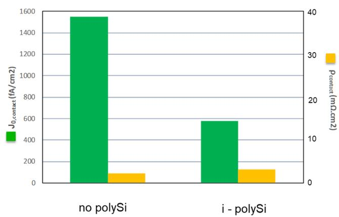
Figure 25. Reduction of  $J_{0,contact}$  while keeping low  $R_{contact}$  when inserting an intrinsic polysilicon layer under the emitter contact.
