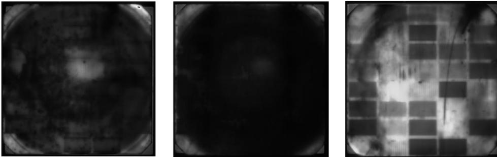
Figure 9. PL images of samples diffused at 1000, 925, and 900°C showing ring patterns indicating severe damage to the bulk. (Rectangular shapes are from defined test patterns applied on the samples).
