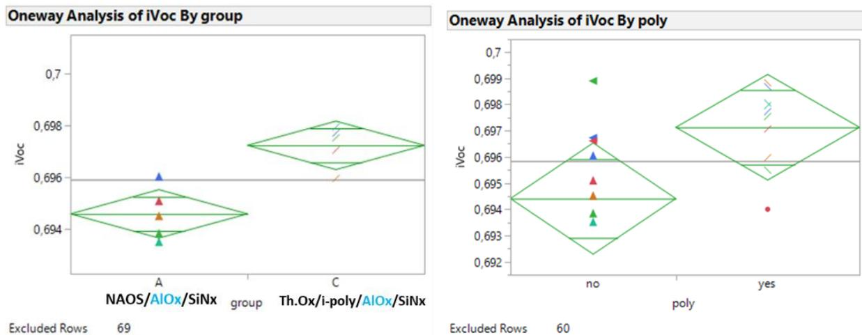
Figure 5. Detailed statistical analysis comparing distinct selections of the experiment, showing significant improvement of emitter passivation by the insertion of an intrinsic polysilicon layer between the emitter and the dielectric layers.
