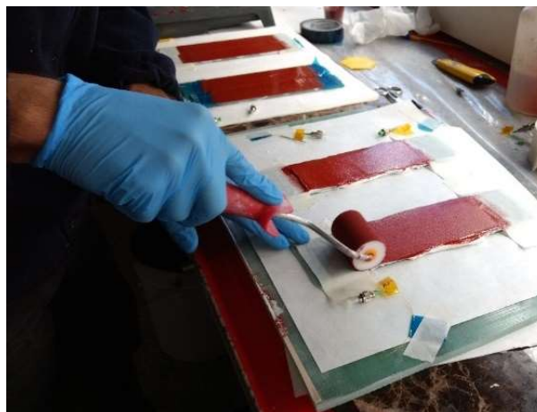
Figure 7 - Incorporation of TNO sensor fibres in Aerox coatings at Aerox laboratories Valencia.
