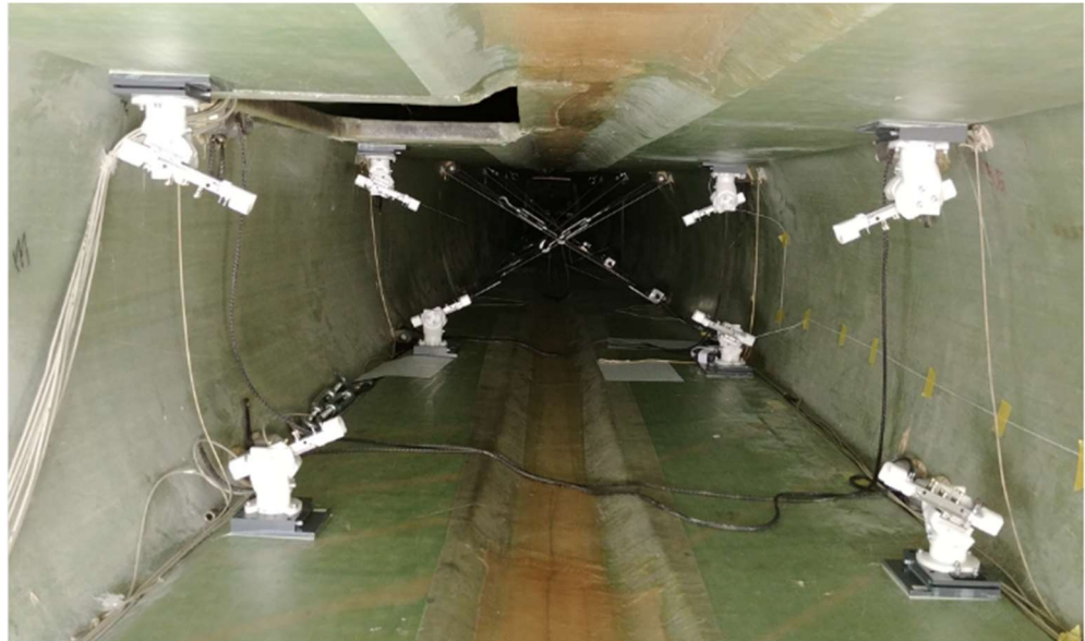
Figure 2 - CSSDS test integration at DTU, installed FCMs inside the blade (left) and test rig (right)
