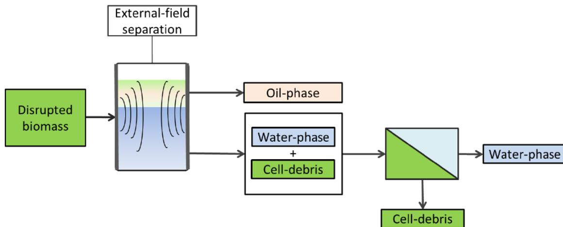
**Figure 3. Illustration of separation of the hydrophobic (lipid) phase from the aqueous phase using external fields.**
