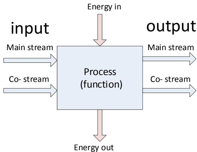
*Figure 7 Representation of the process units and properties of energy and mass streams into and out of the system. The main stream contains the algal biomass or the aimed components, the co-stream the required additional components or emitted products.*
