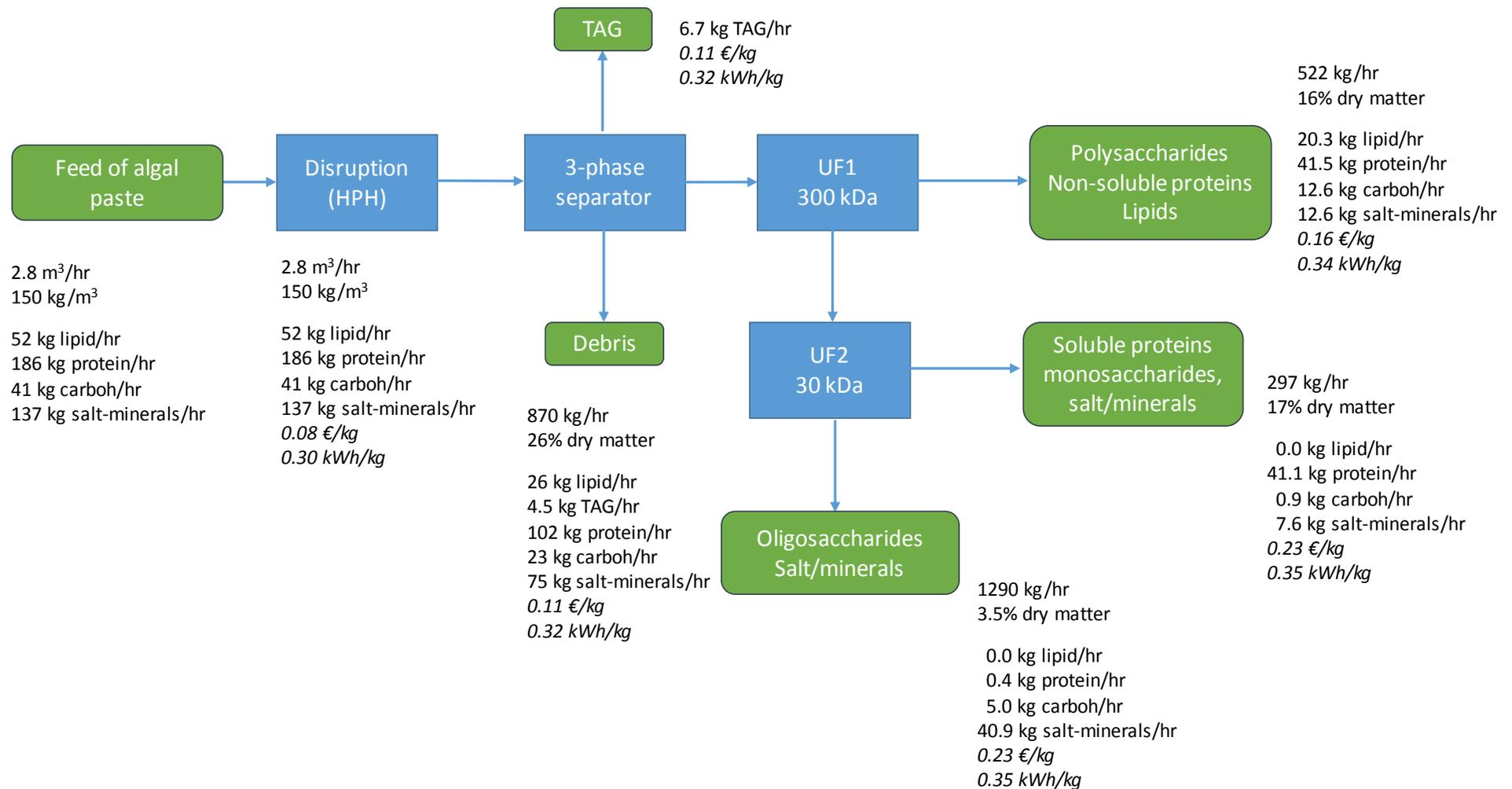
**Figure 12 Soluble component fractionation from 3-phase centrifugal separation for homogenized non-stressed algae with component mass balances and estimated allocated costs and energy consumption for each product (italic)**
