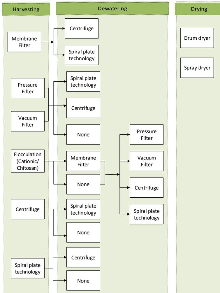
**Figure 8** Combination of operations for harvesting and dewatering of algal biomass at large scale.
