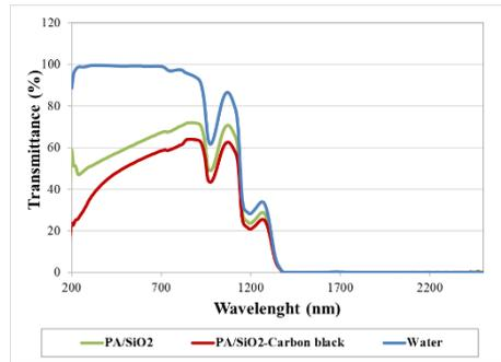
**Fig. 2** Transmittance spectra of PA/SiO<sub>2</sub>-carbon black slurries
