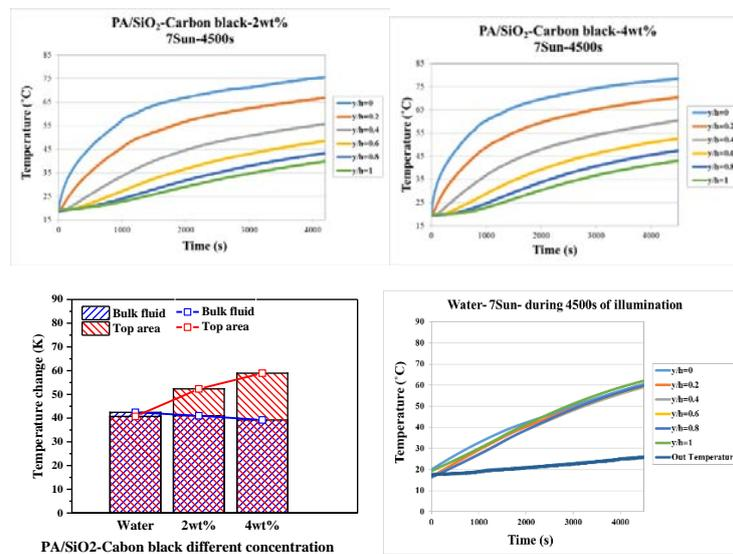
Fig. 4 Photo-thermal performance of different concentrations of PA/SiO<sub>2</sub>-Carbon black slurries
