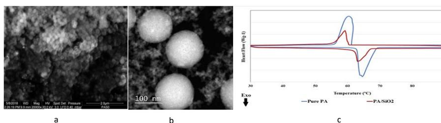
**Fig. 1** from left to right: a) SEM, b) HAADF-STEM and c) DSC outcomes of PA/SiO<sub>2</sub> SSPCMs
