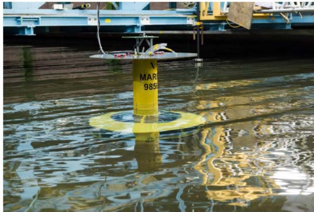
Figure 6-5: Model tests for the installation of a GBS as part of the GBS WIND JIP
