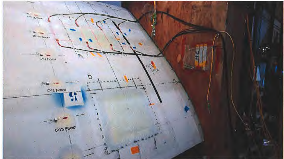
Figure 8. A photo of the section of the wind turbine blade at WMC, with all the installed sensors of TNO, UT and WMC.
