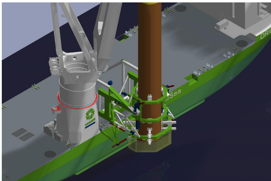
Figure 2-1, Basic design of the Motion Compensated Pile Gripper
