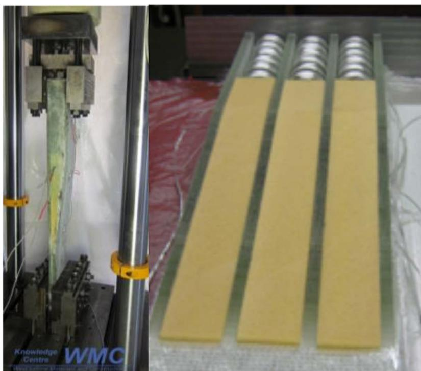
Figure 32: Test on rotor blade insert (left) and insert details (right)
