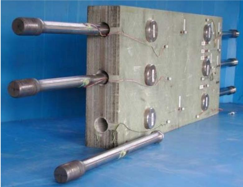
Figure 29: Typical T-bolt test specimen (WMC)
