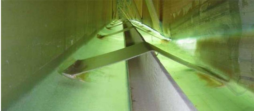
**Figure 43: Bladena cap stiffener, to facilitate spar cap reduction**
