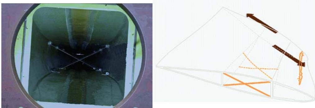
**Figure 42: X-stiffener, to avoid longitudinal bondline cracks due to cross-sectional shear distortion [45]**
