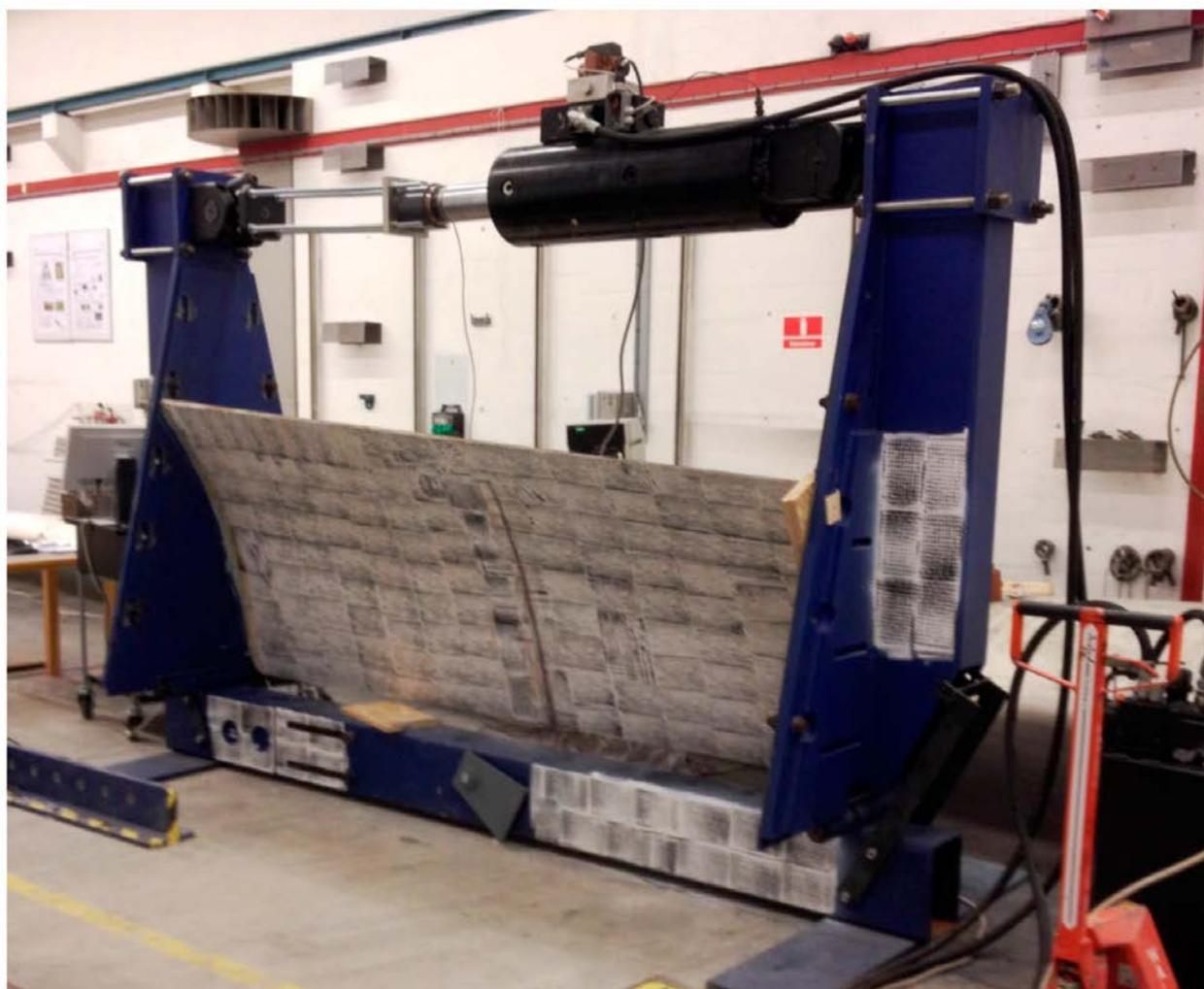
**Figure 4: Test set-up for trailing edge buckling at DTU [5]**
