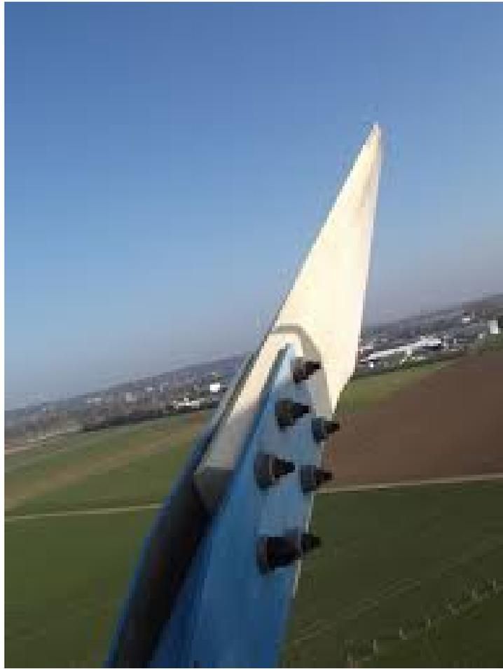
Figure 25: clamped root
