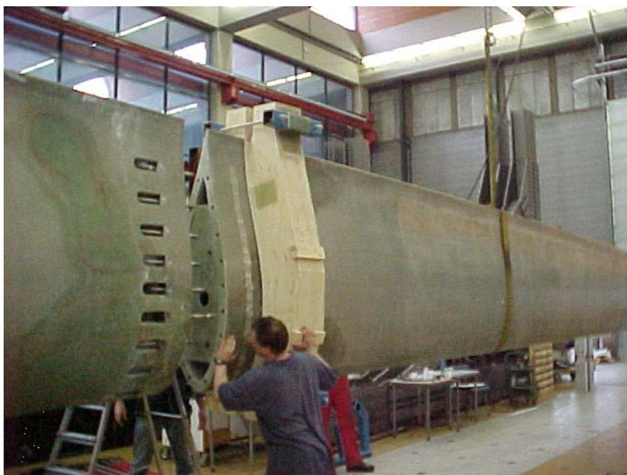
**Figure 8: preparation of a full-scale 23.3m blade test**
