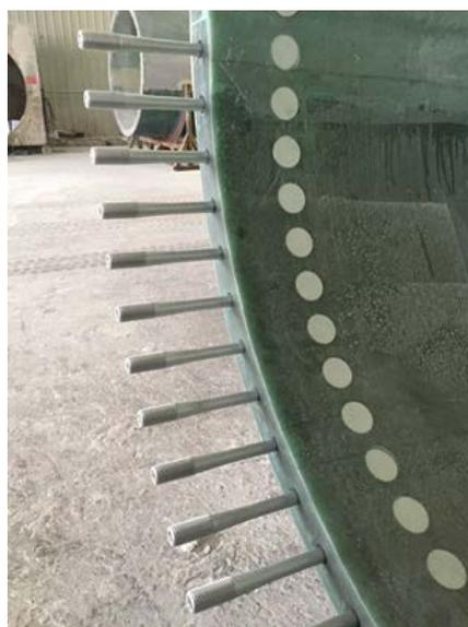
**Figure 28: T-bolt blade root connection (TRES4) [29]**
