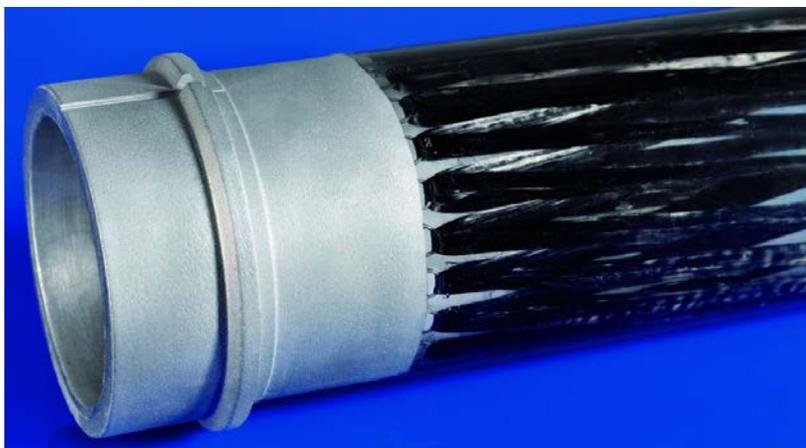
Figure 38: Hybrid connection between Aluminium part and carbon fibres using titanium loops [40]
