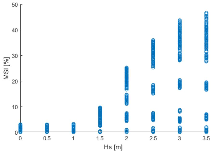
Figure 12 Motion sickness incidence versus significant wave height for 84-metre SOV
