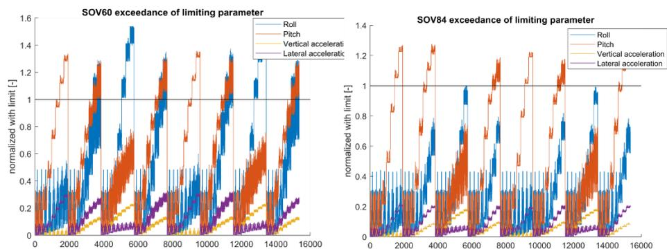
Figure 8 Exceedance of limit for all entries in the hydrodynamic database (limit given in root mean square, response parameter as standard deviation)
