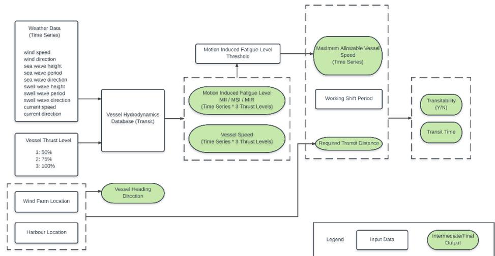
Figure 4 Illustration of the new approach to assess the vessel transitability and transit time
