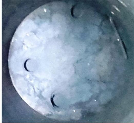
Figure 6. Hard carbon layer found in pre-reformer reactor after test in January 2017.
